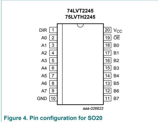
Figure 4. Pin configuration for SO20
