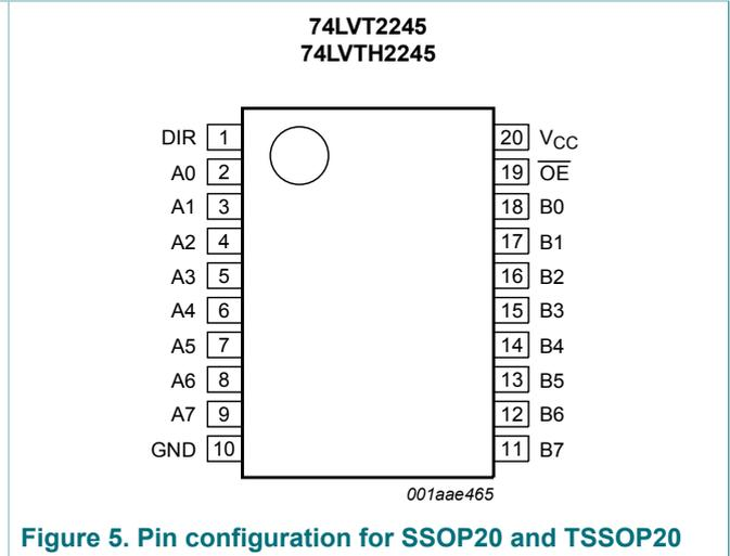
Figure 5. Pin configuration for SSOP20 and TSSOP20
