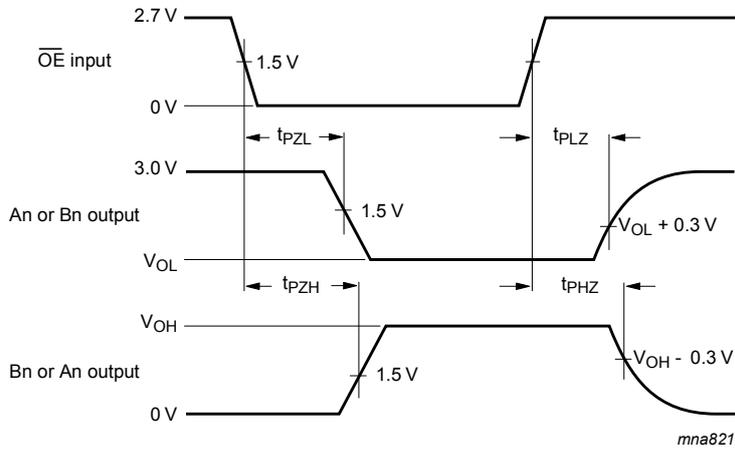
$V_{OL}$  and  $V_{OH}$  are typical voltage output levels that occur with the output load.
