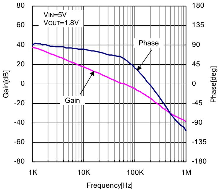
Figure 25. Closed Loop Response (VIN=5V, VOUT=1.8V, IOUT=1A, L=1.5μH, COUT=Ceramic 44μF)
