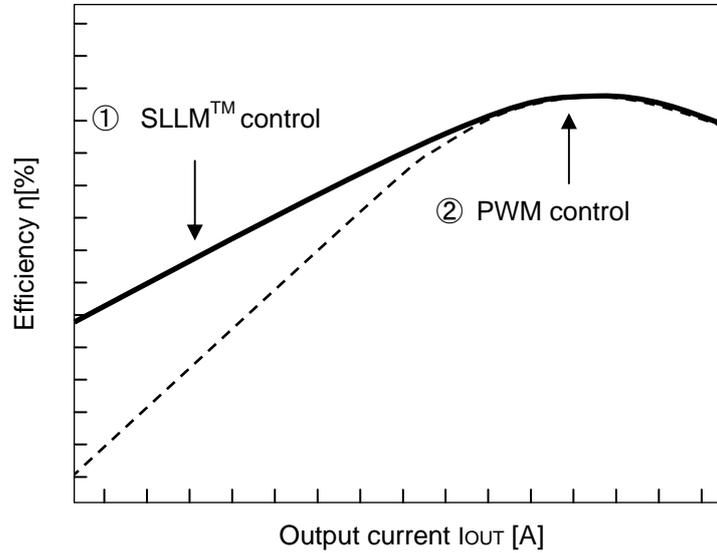
Figure 41. Efficiency (SLLM™ control and PWM control)
