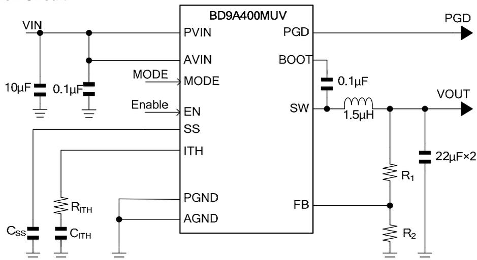
Figure 1. Application Circuit
