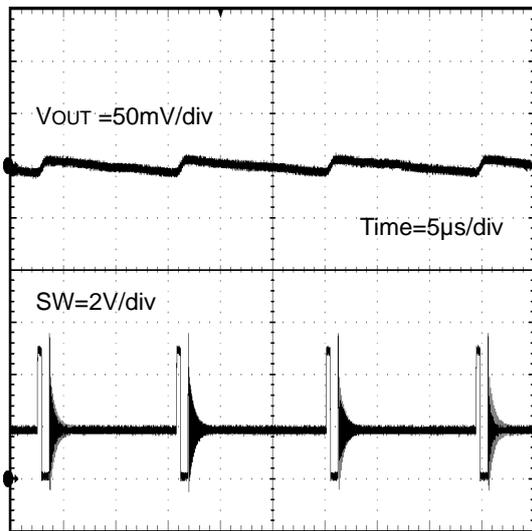
Figure 42. SW Waveform (SLLM™ control)
