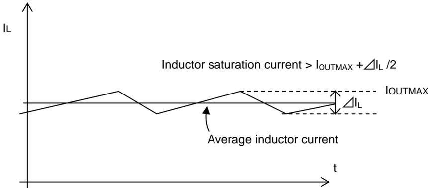
Figure 49. Waveform of current through inductor
