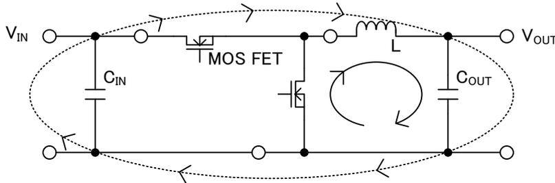
Figure 54. Current Loop of Buck DC/DC Converter
