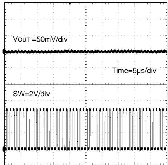
Figure 43. SW Waveform (PWM control)
