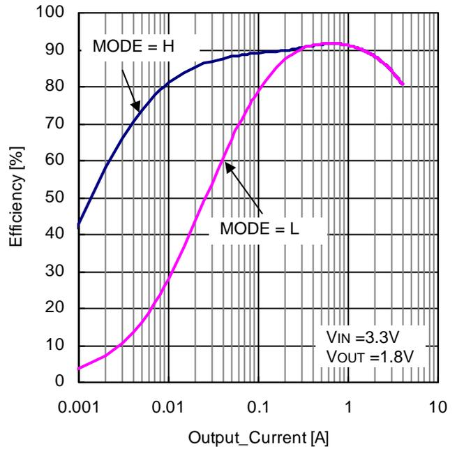
Figure 23. Efficiency vs Load Current (VIN=3.3V, VOUT=1.8V, L=1.5μH)
