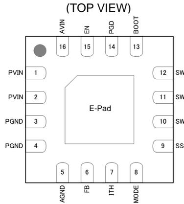
Figure 2. Pin Configuration
