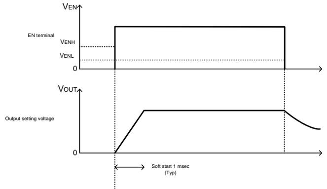
Figure 44. Start Up and Down with Enable
