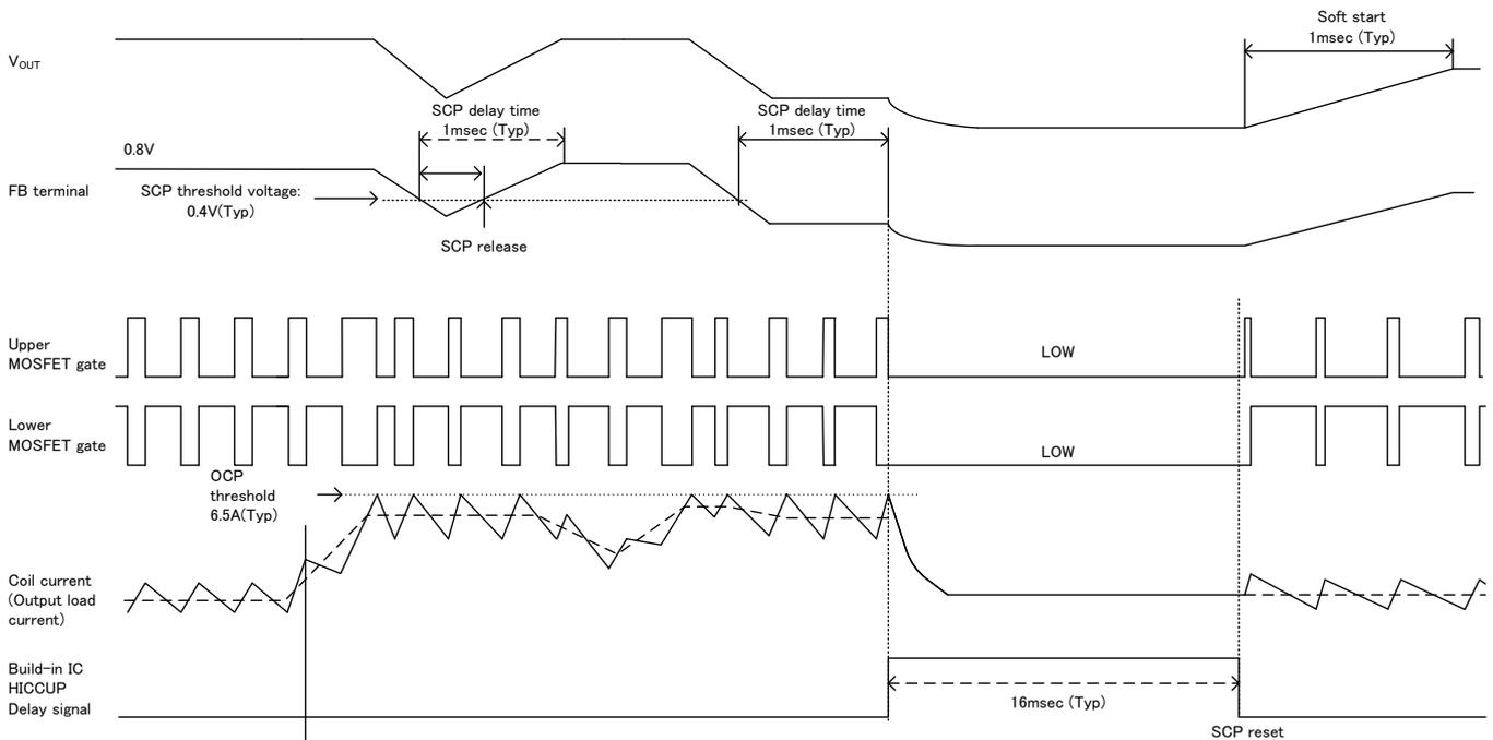
Figure 46. Short Circuit Protection (SCP) timing chart
