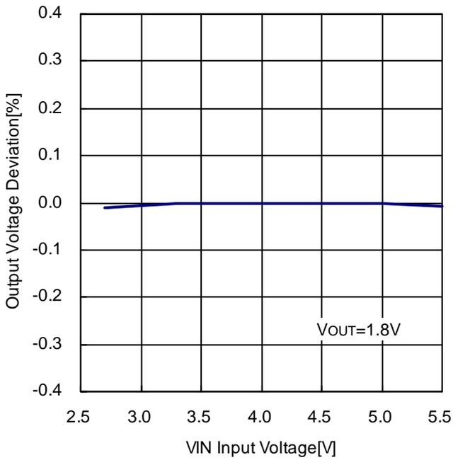
Figure 37. Line Regulation vs Input Voltage
