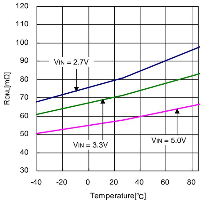
Figure 15. Low side FET ON-Resistance vs Temperature
