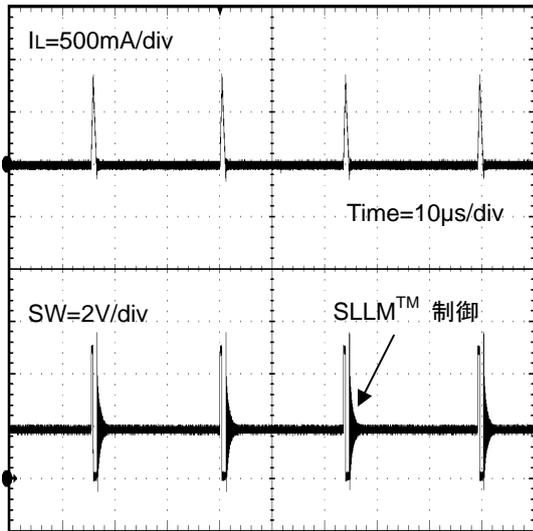
Figure 36. Switching Waveform with SLLM™
