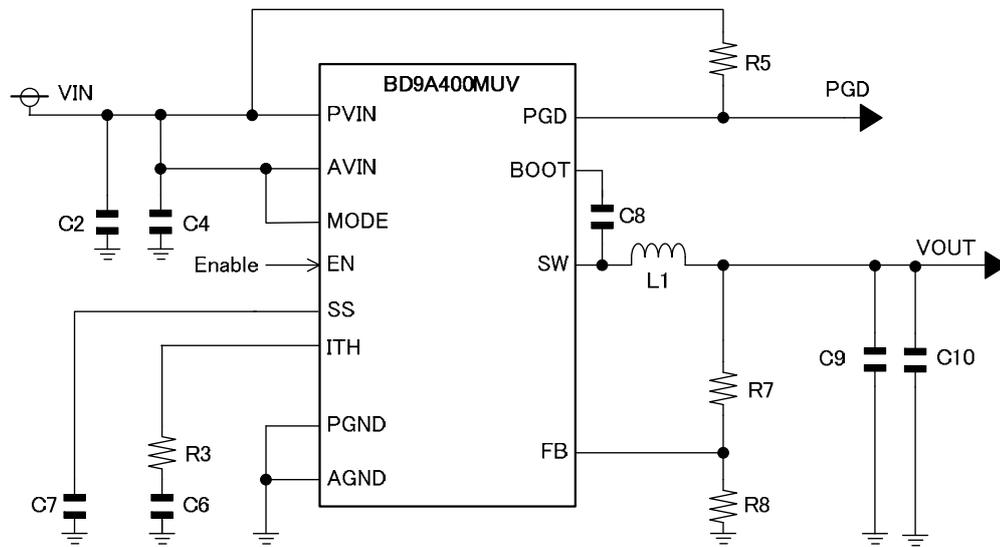
Figure 48. Application Circuit
