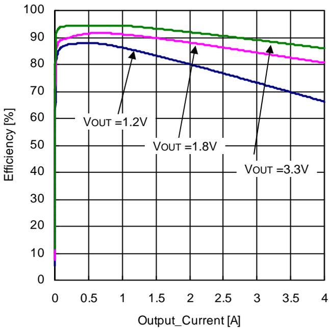
Figure 24. Efficiency vs Load Current (VIN = 5.0V, MODE = 5.0V, L=1.5μH)
