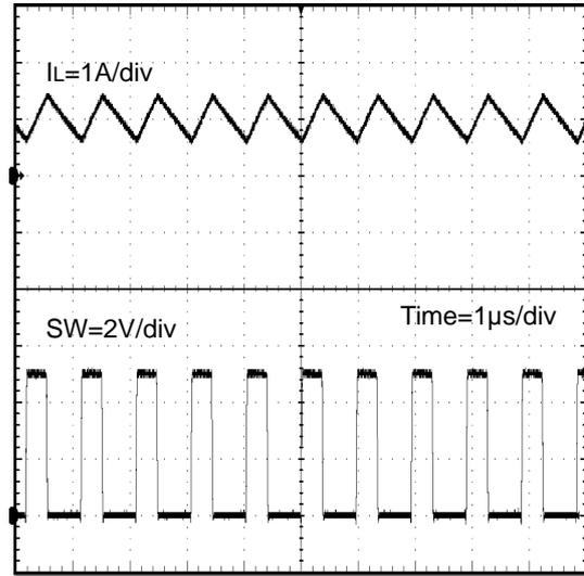
Figure 35. Switching Waveform
