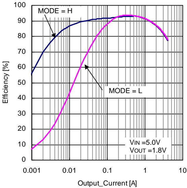
Figure 22. Efficiency vs Load Current (VIN=5V, VOUT=1.8V, L=1.5μH)
