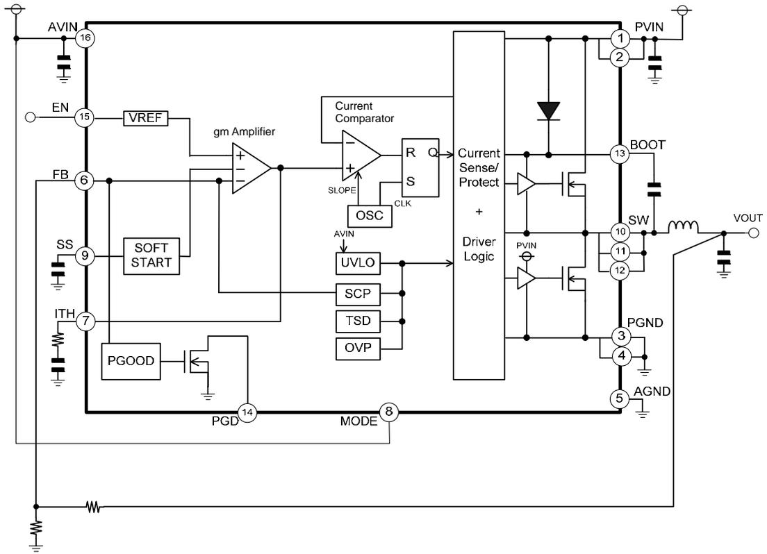
Figure 3. Block Diagram
