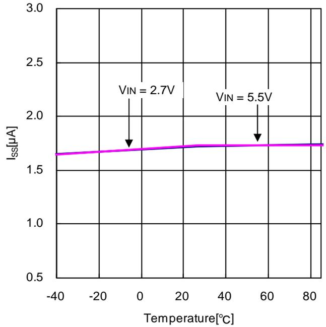
Figure 13. Soft Start Terminal Current vs Temperature
