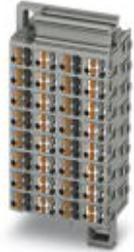
Marshalling patchboard, Nom. voltage: 500 V, Nominal current: 17.5 A, Cross section: 0.14 mm<sup>2</sup> - 2.5 mm<sup>2</sup>, AWG: 12 - 26, Connection type: Push-in connection, Number of positions: 32, Number of connections: 128, Width: 44 mm, Length: 73.2 mm, Color: gray, Color of connection elements: gray/white, Assembly: Wall mounting
