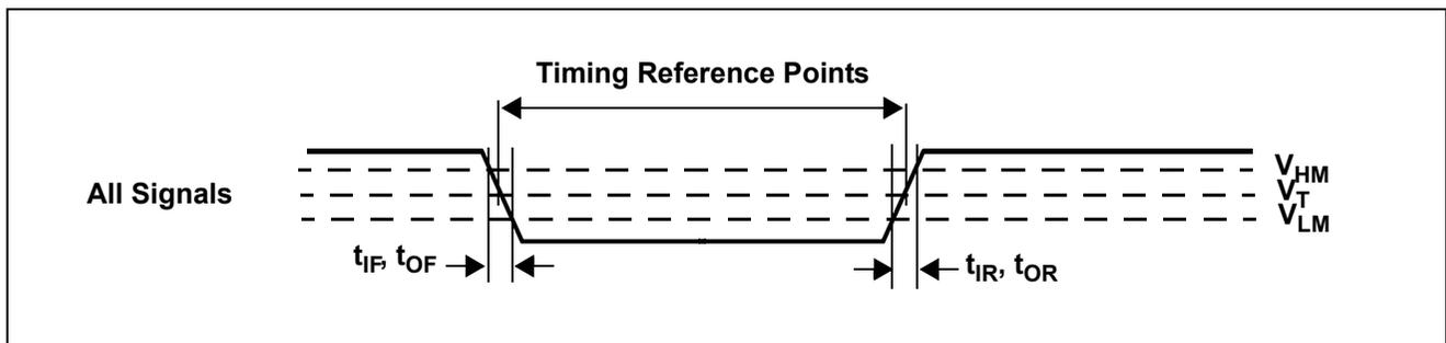
**Figure 11 - Output Timing Parameter Measurement Voltage Levels**
