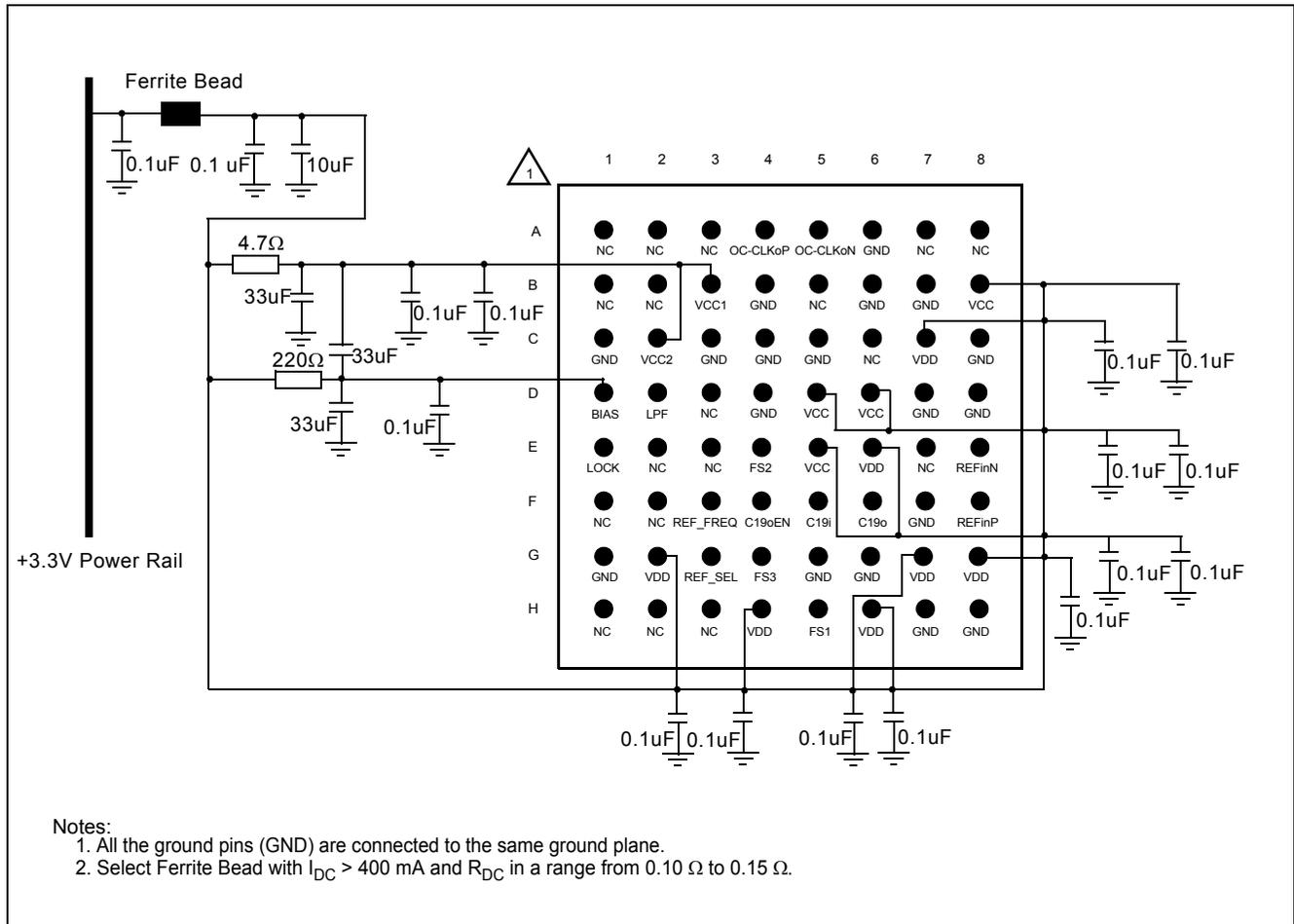
Figure 10 - Power Supply and BIAS Circuit Filtering
