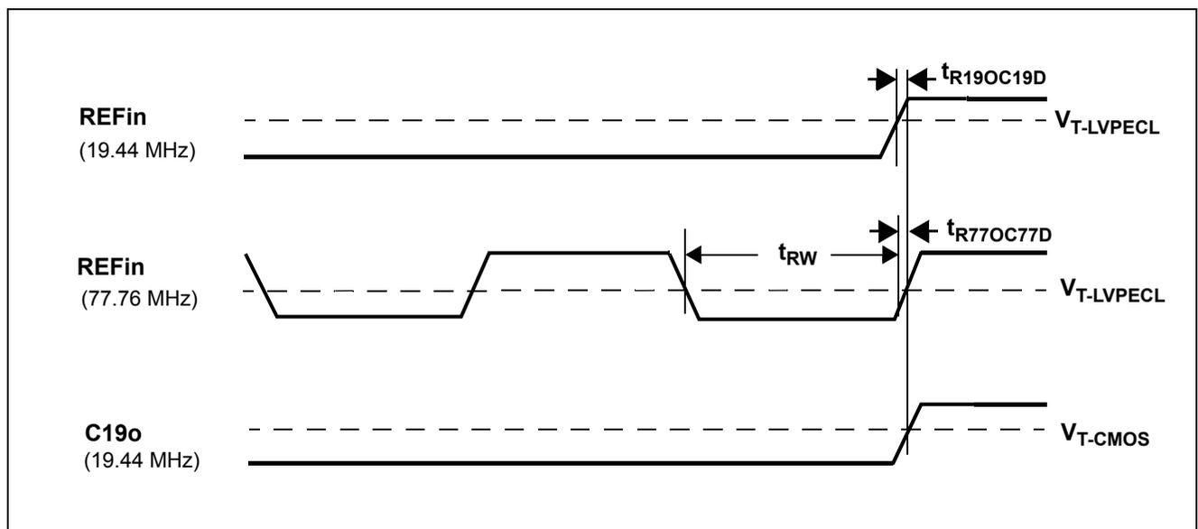
**Figure 13 - REFin Input to C19o Output Timing**
