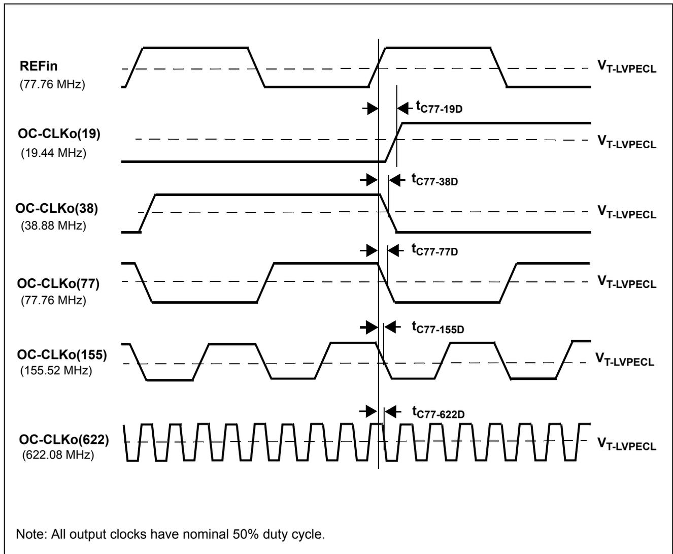
**Figure 16 - REFin (77.76 MHz) Input to OC-CLKo Output Timing**
