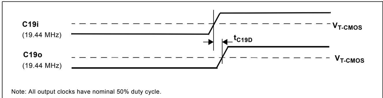
**Figure 12 - C19i Input to C19o Output Timing**
