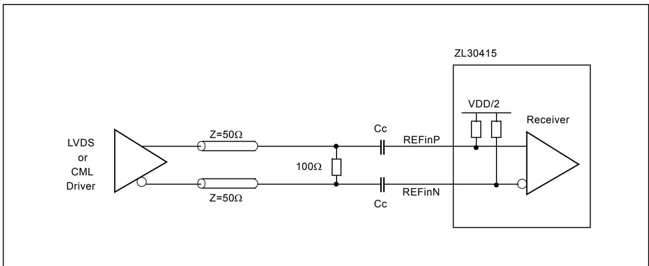
Figure 8 - Interfacing to LVDS or CML Driver
