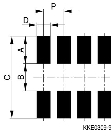
**Recommended dimensions (mm) for reflow soldering**
