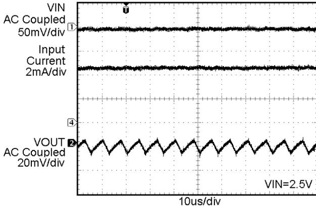
Figure 19. Operating Waveforms in 1.5x Mode
