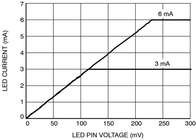
Figure 4. LED Current vs. LED Pin Voltage
