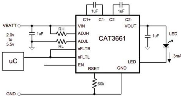
**Figure 25. Application Circuit with  $R_H$  &  $R_L$**
