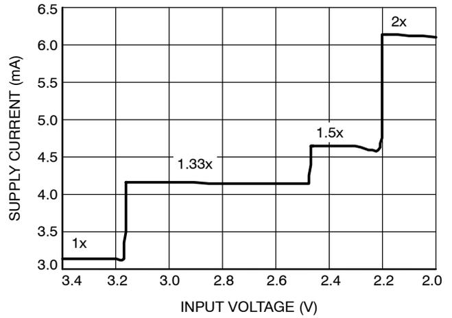
Figure 3. Total Supply Current vs. Input Voltage
