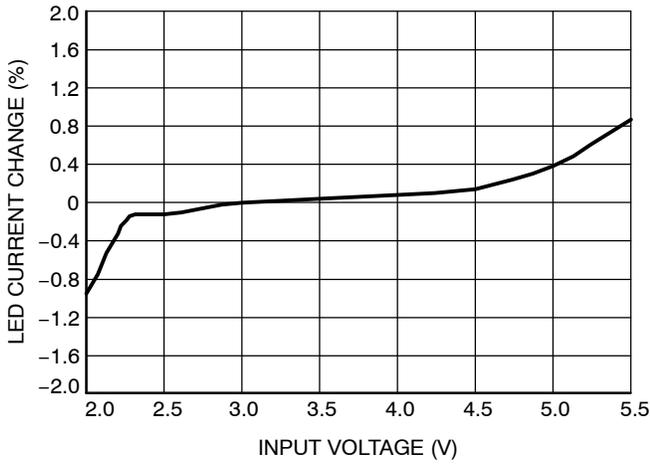
Figure 9. LED Current Change vs. Input Voltage
