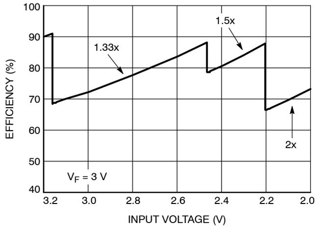
Figure 12. Efficiency vs. Lithium Coin Cell Voltage
