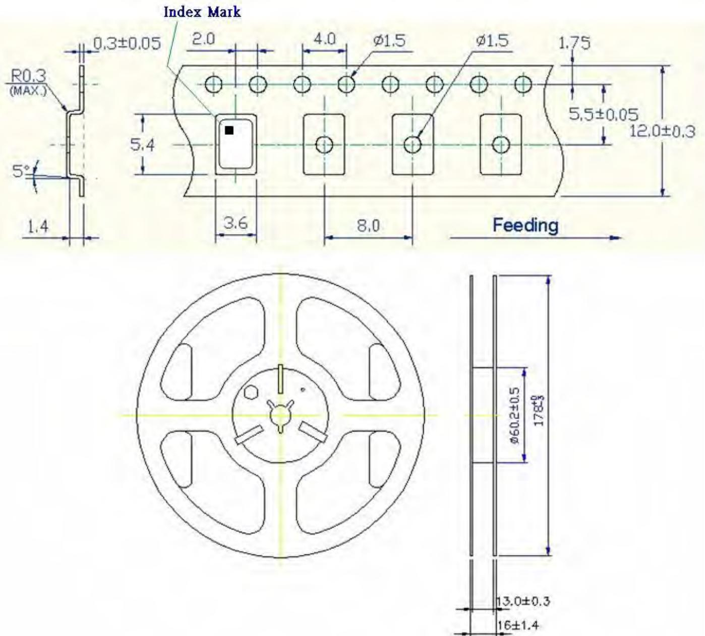
1. 230mm minimum leader which consist of carrier and/or tape followed by a minimum of 160mm of empty carrier tape sealed with cover tape.
