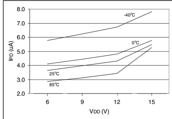
**FIGURE 11-8: MAXIMUM I<sub>PD</sub> vs. VDD, WATCHDOG TIMER ENABLED (V<sub>IO</sub> = 5V)**
