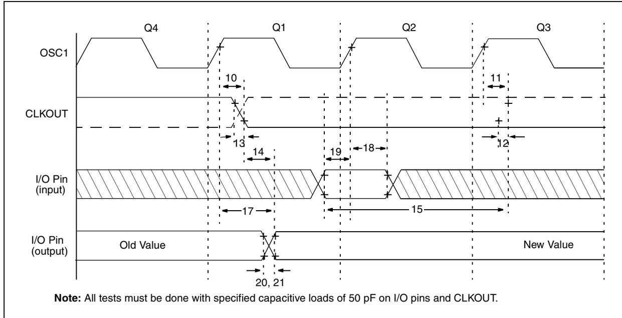
**TABLE 10-2: CLKOUT AND I/O TIMING REQUIREMENTS - PIC16HV540**
