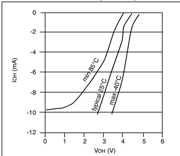
**Note:** Current being applied is being applied simultaneously to all 4 PORTA pins.
