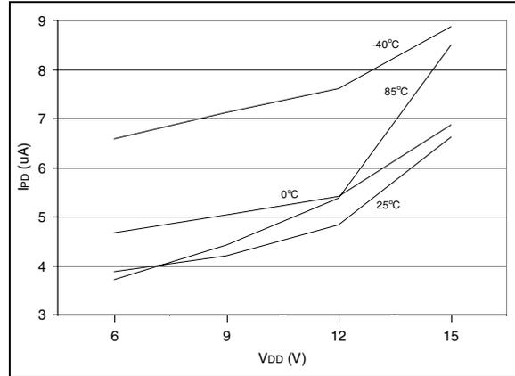
**FIGURE 11-9: TYPICAL I<sub>PD</sub> vs. VDD, WATCHDOG TIMER DISABLED (V<sub>IO</sub> = 3V)**
