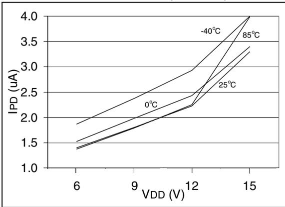
**FIGURE 11-6: MAXIMUM I<sub>PD</sub> vs. VDD, WATCHDOG TIMER DISABLED (V<sub>IO</sub> = 5V)**
