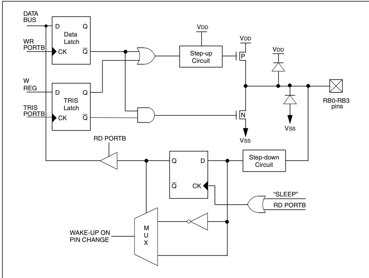
**FIGURE 5-3: BLOCK DIAGRAM OF PORTB<4:6> PINS**
