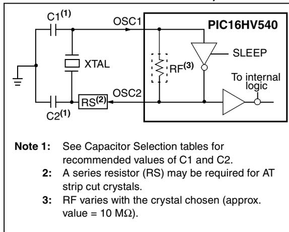
**FIGURE 7-2: EXTERNAL CLOCK INPUT OPERATION (HS, XT OR LP OSC CONFIGURATION)**
