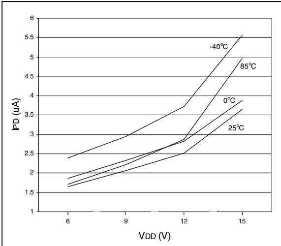
**FIGURE 11-7: TYPICAL I<sub>PD</sub> vs. VDD, WATCHDOG TIMER ENABLED (V<sub>IO</sub> = 5V)**
