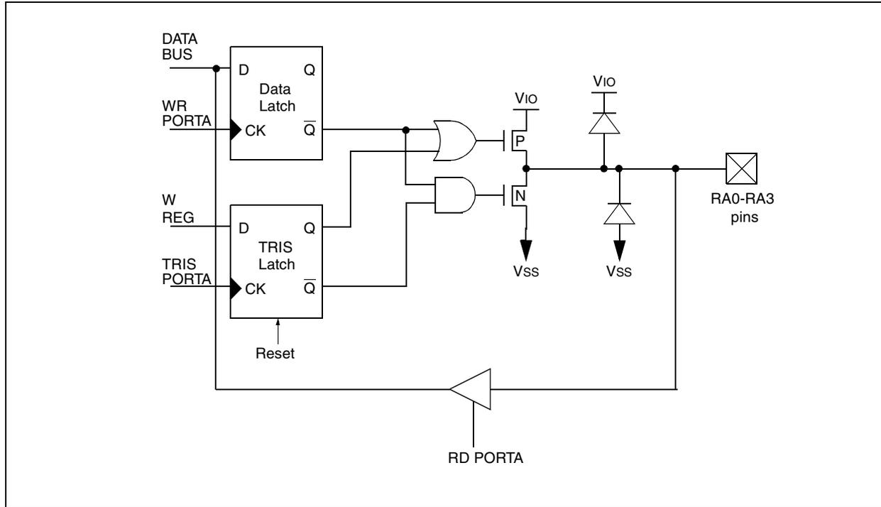
**FIGURE 5-2: BLOCK DIAGRAM OF PORTB<0:3> PINS**
