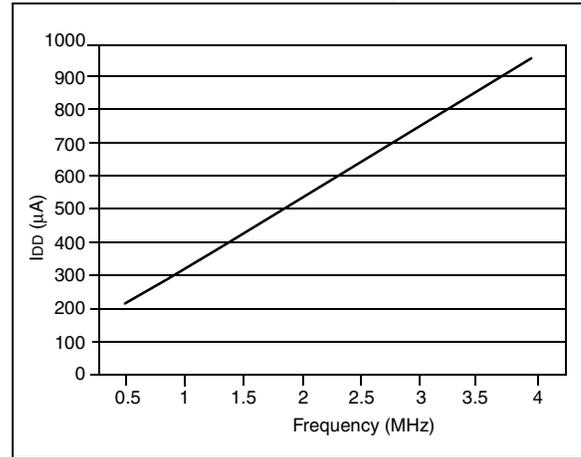
**FIGURE 11-14: MAXIMUM IDD vs. FREQUENCY, WATCHDOG TIMER ENABLED, RC MODE (VDD = 15V, VIO = 5V)**
