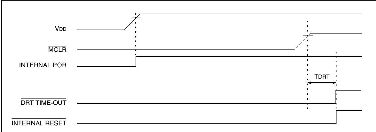
**FIGURE 7-9: TIME-OUT SEQUENCE ON POWER-UP ( $\overline{\text{MCLR}}$  TIED TO  $V_{\text{DD}}$ ): FAST  $V_{\text{DD}}$  RISE TIME**
