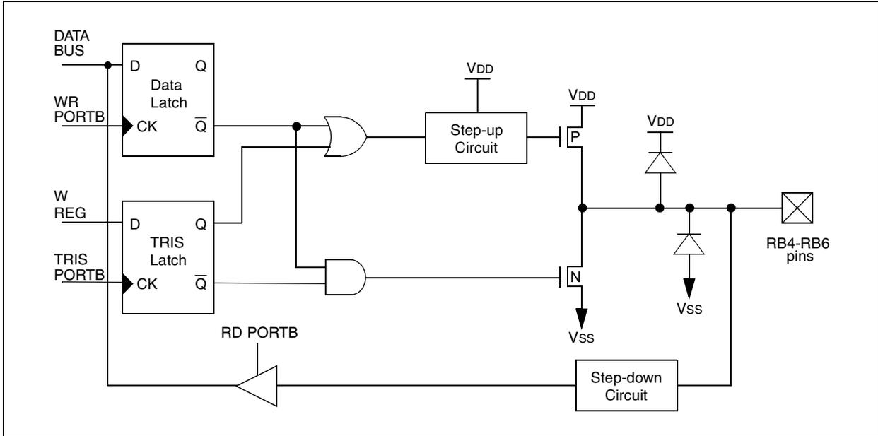
**FIGURE 5-4: BLOCK DIAGRAM OF PORTB<7> PIN**
