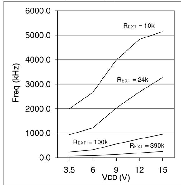
**FIGURE 11-3: TYPICAL RC OSCILLATOR FREQUENCY vs. VDD (C<sub>EXT</sub> = 100pF)**
