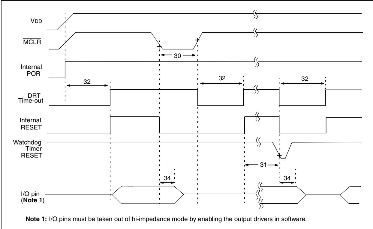
FIGURE 10-5: BROWN-OUT DETECT TIMING
