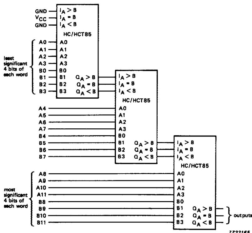
Fig.7 Series cascading; comparing 12-bit words.
