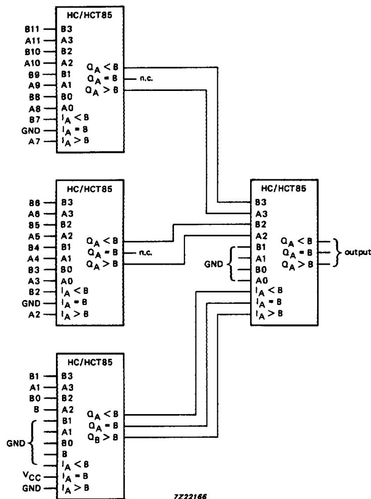
Fig.8 Parallel cascading; comparing 12-bit words.
