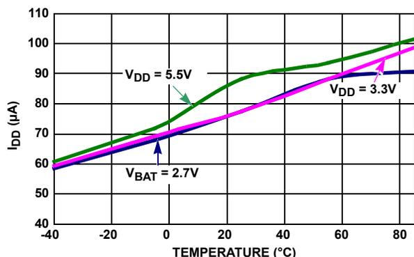
FIGURE 11.  $I_{DD}$  with TSE = 1 vs TEMPERATURE
