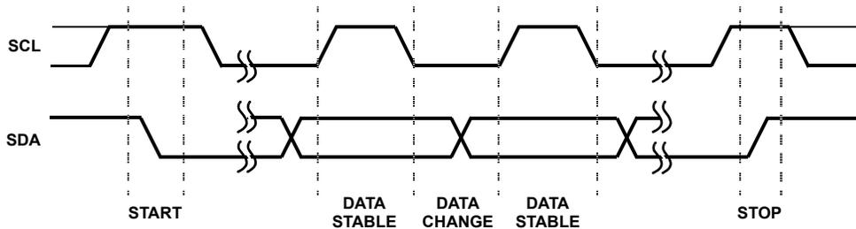
FIGURE 16. VALID DATA CHANGES, START AND STOP CONDITIONS
