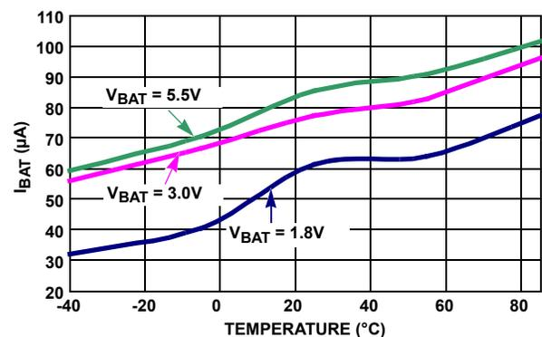
FIGURE 10.  $I_{BAT}$  WITH  $TSE = 1$ ,  $BTSE = 1$  vs TEMPERATURE
