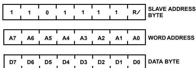
FIGURE 19. SLAVE ADDRESS, WORD ADDRESS AND DATA BYTES
