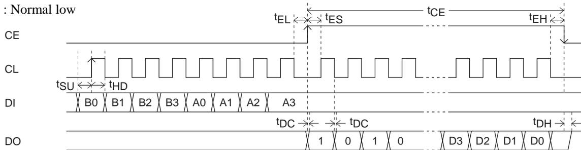
Cautions : 1. Since the DO pin is an n-channel open-drain output, the transition times ( $t_{DC}$ ,  $t_{DH}$ ) will differ with the value of the pull-up resistor used.
