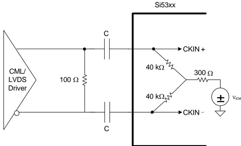
**Figure 38. CML/LVDS Termination (1.8, 2.5, 3.3 V)**
