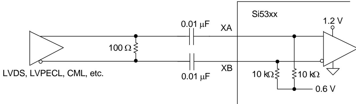
**Figure 51. Differential External Reference Input Example
