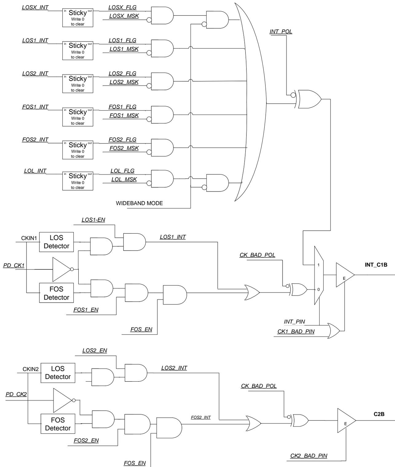
Figure 82. Si5324 and Si5326 Alarm Diagram
