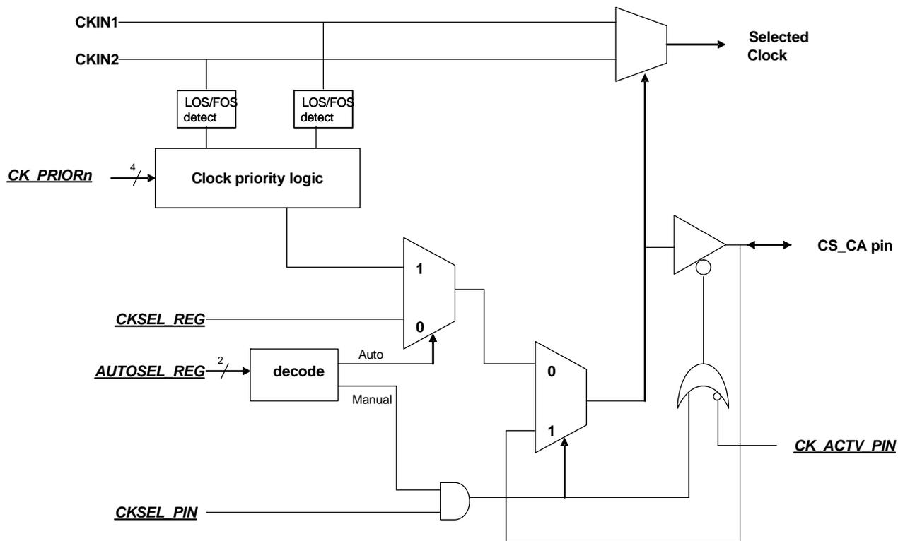
Figure 24. Si5324, Si5325, Si5326, Si5327, Si5374, and Si5376 Input Clock Selection
