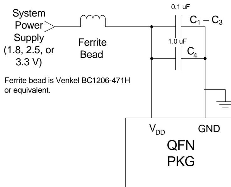
Figure 56. Typical Power Supply Bypass Network (QFN Package)
