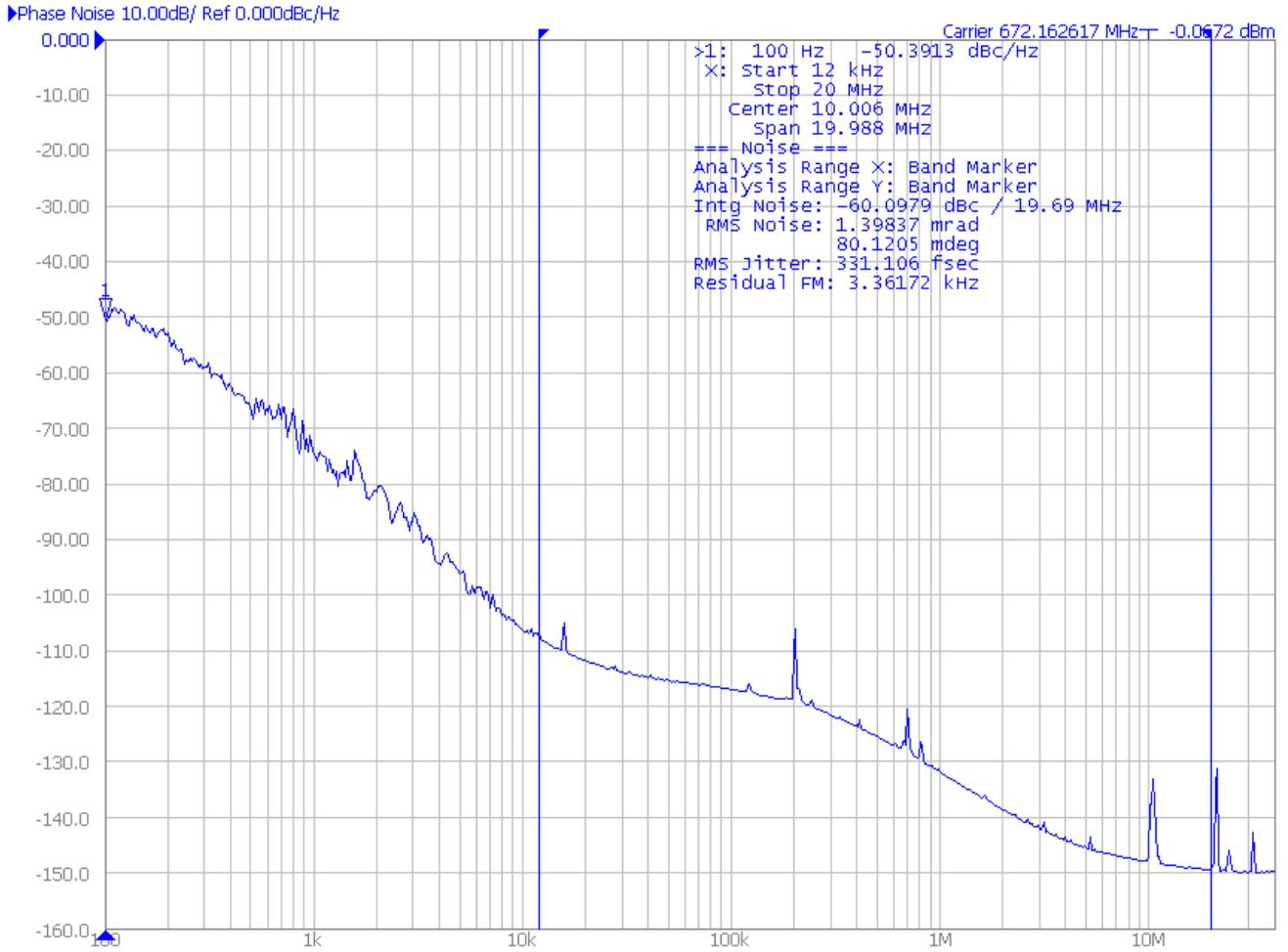
Figure 71. 622.08 MHz In; 672.16 MHz Out; Loop BW = 6.9 kHz
