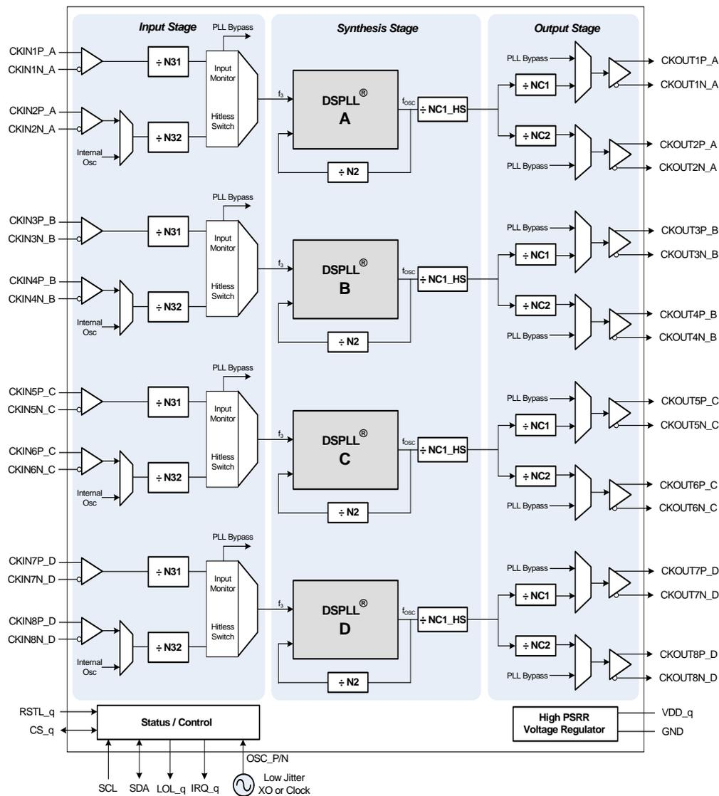
Figure 16. Si5376 Functional Block Diagram
