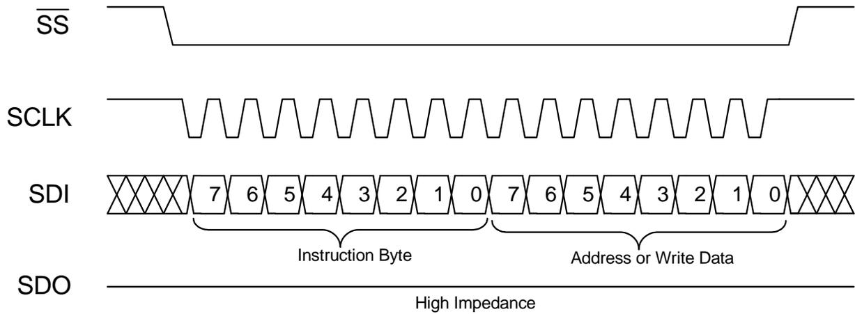
**Figure 33. SPI Write/Set Address Command**
