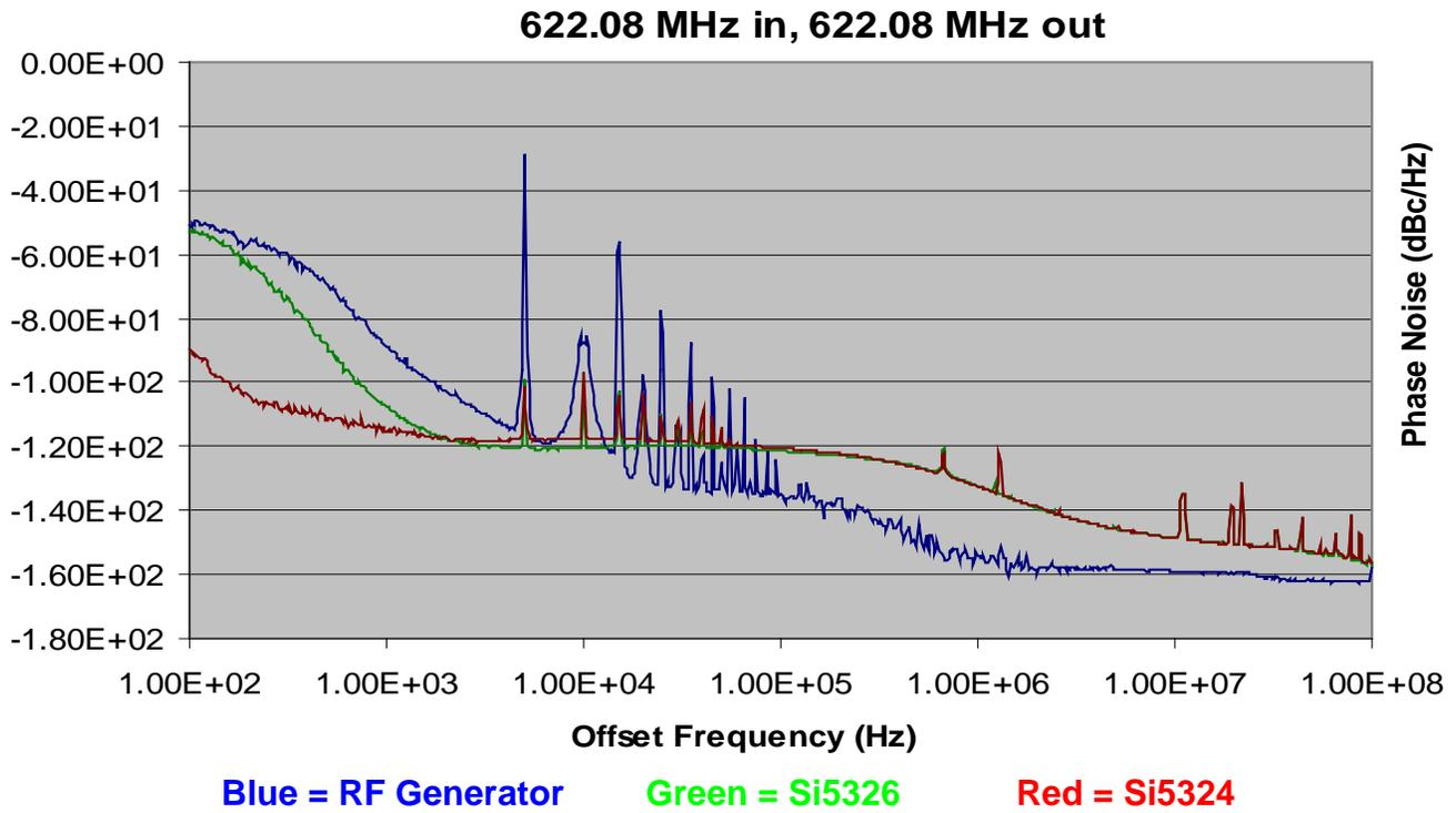
Figure 93. RF Generator, Si5326, Si5324 (5 kHz Jitter)
