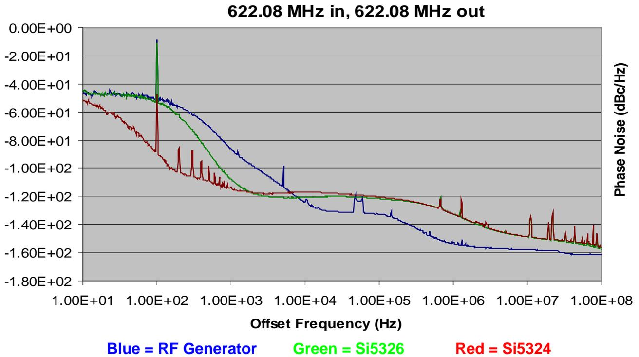
Figure 90. RF Generator, Si5326, Si5324 (100 Hz Jitter)
