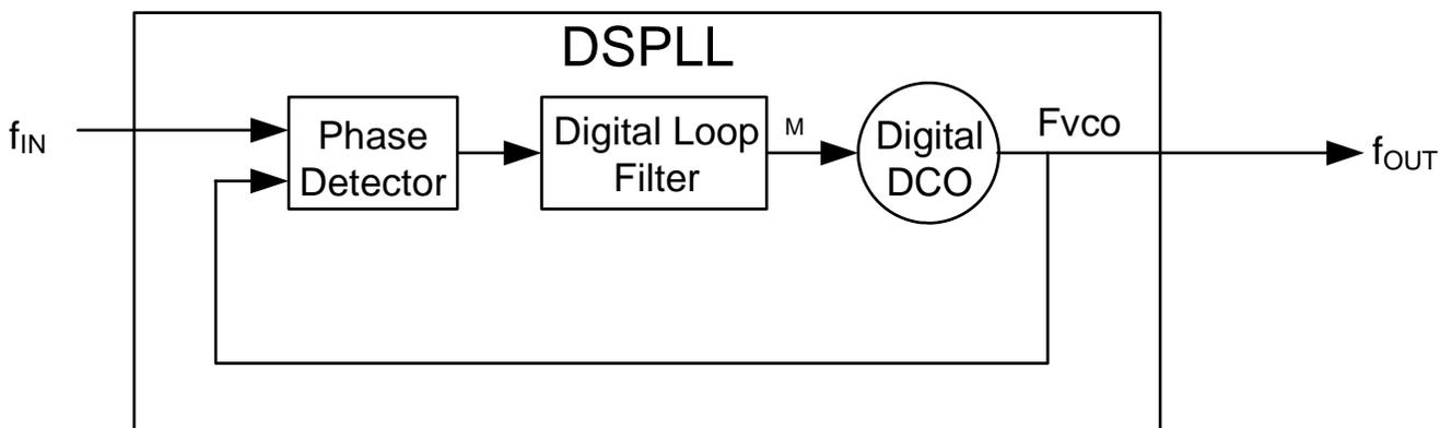
Figure 17. Any-Frequency Precision Clock DSPLL Block Diagram
