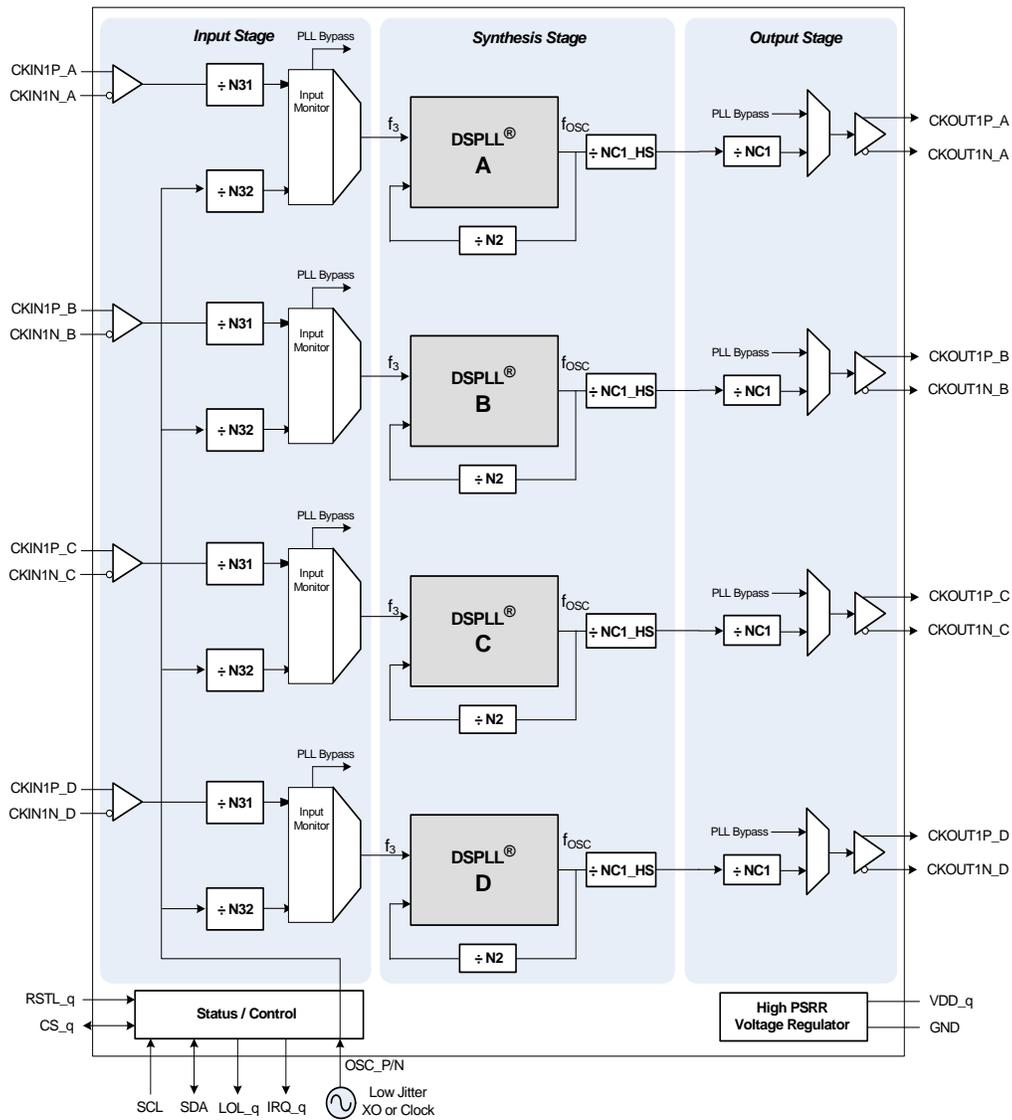
Figure 15. Si5375 Functional Block Diagram
