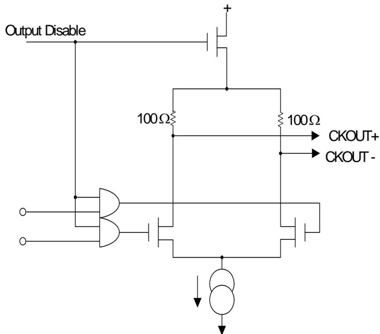
**Figure 43. Differential CKOUT Structure (not for CMOS)**
