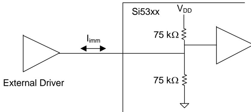
Figure 53. Three Level Input Pins
