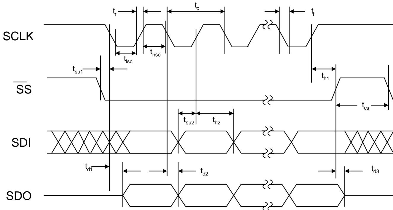
Figure 35. SPI Timing Diagram
