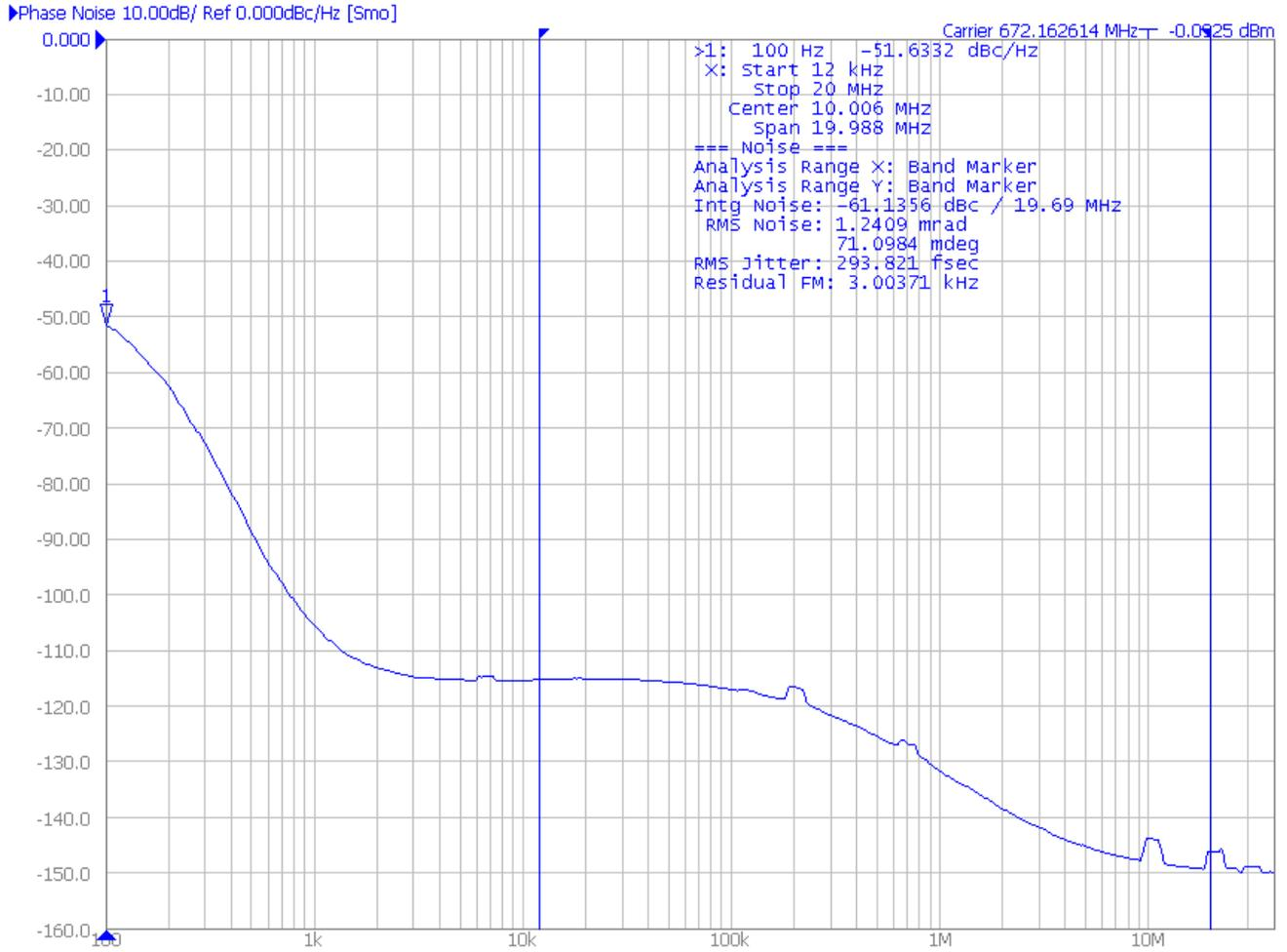
Figure 72. 622.08 MHz In; 672.16 MHz Out; Loop BW = 100 Hz
