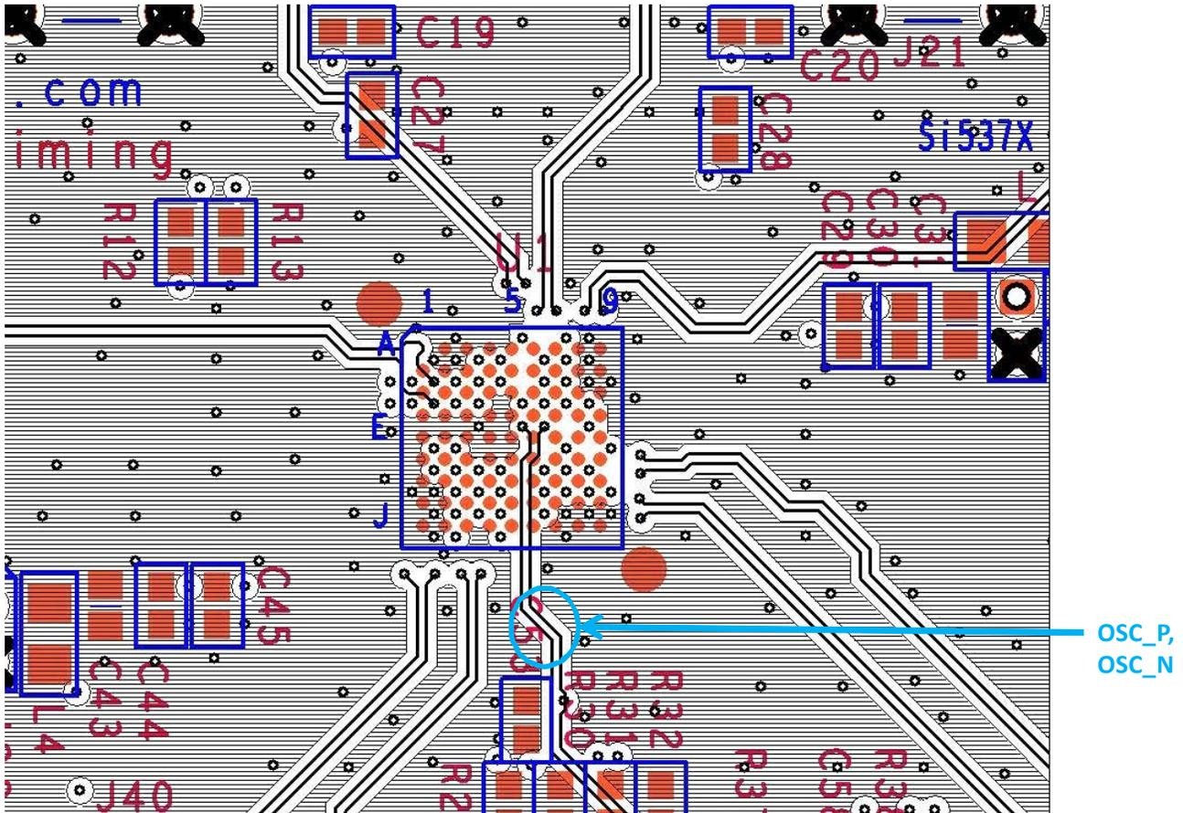
Avoid placing the OCS\_P and OSC\_N signals on the same layer as the clock outputs. Add grounded guard traces surrounding the OSC\_P and OSC\_N signals.
