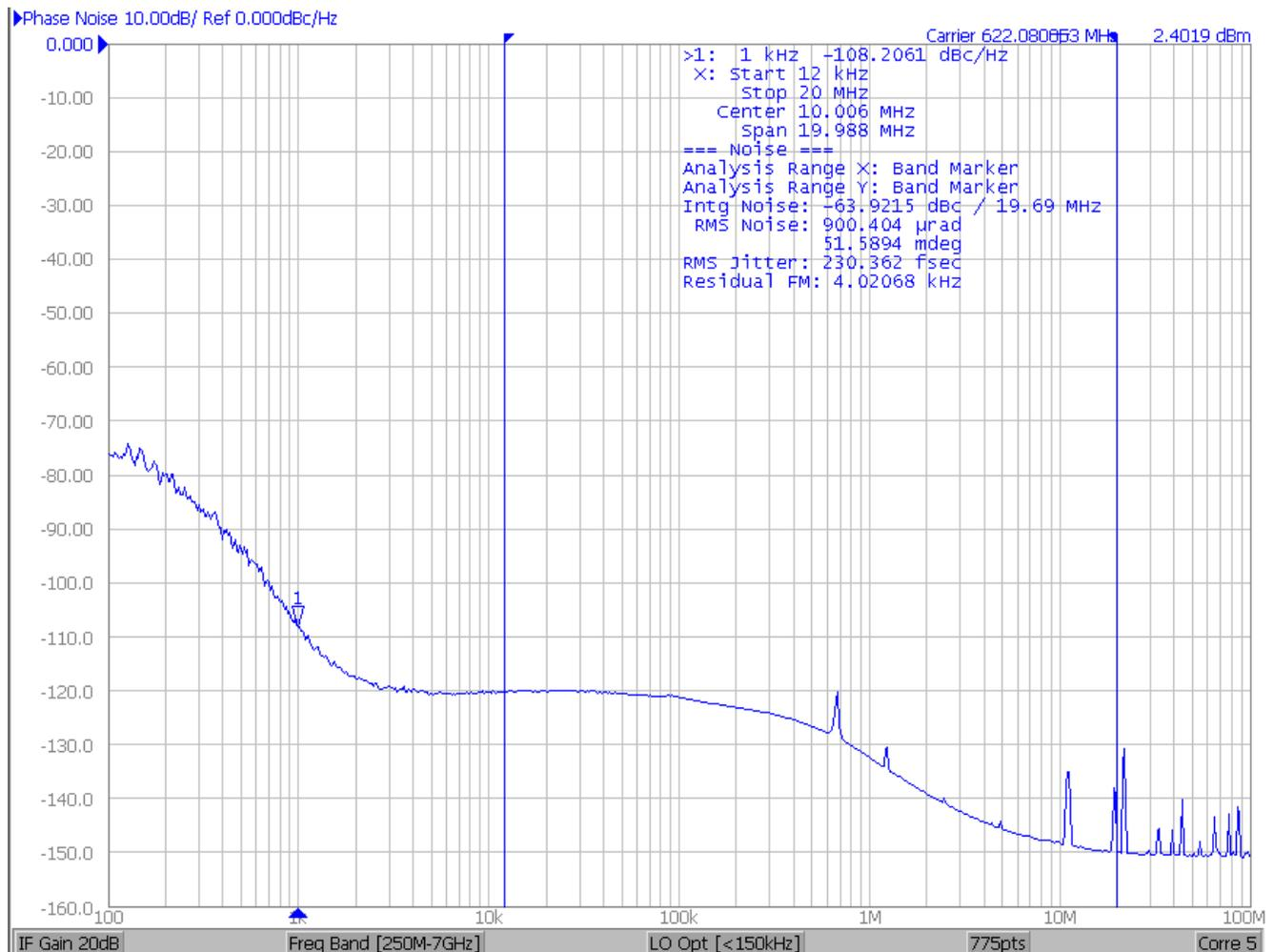
Figure 63. 622.08 MHz Output with a 114.285 MHz Crystal
