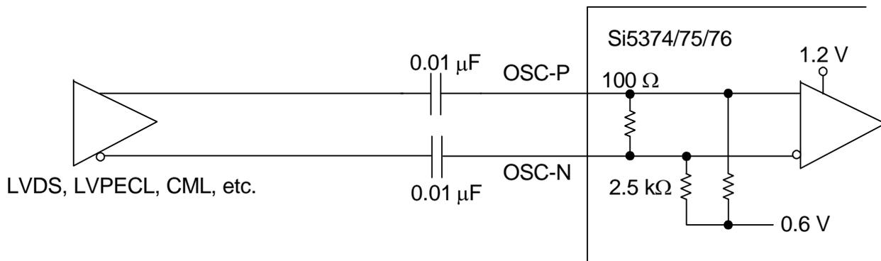
**Figure 52. Differential OSC Reference Input Example for Si5374, Si5375 and Si5376**
