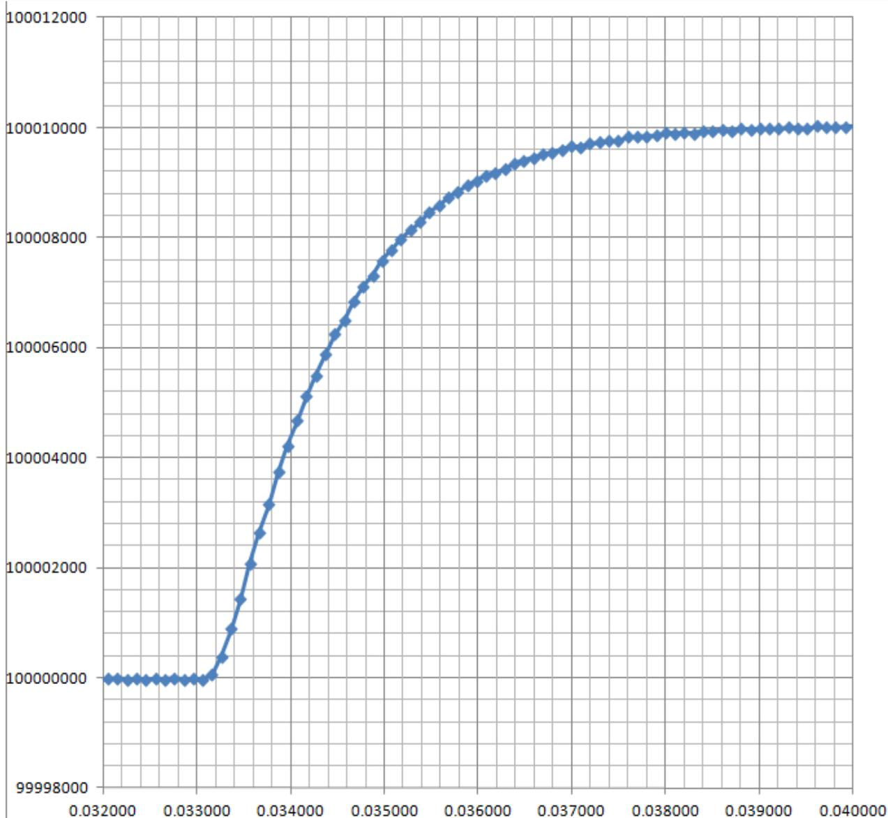
Figure 95. Si5326 Frequency Step Function Response
