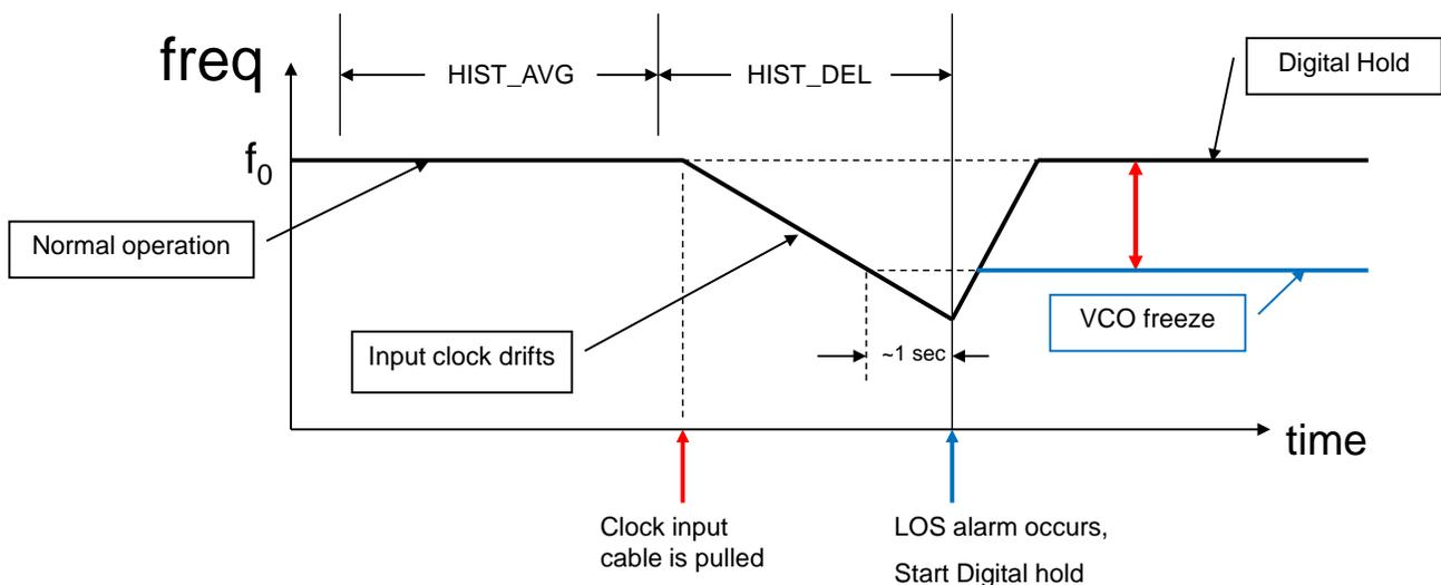
Figure 28. Digital Hold vs. VCO Freeze Example
