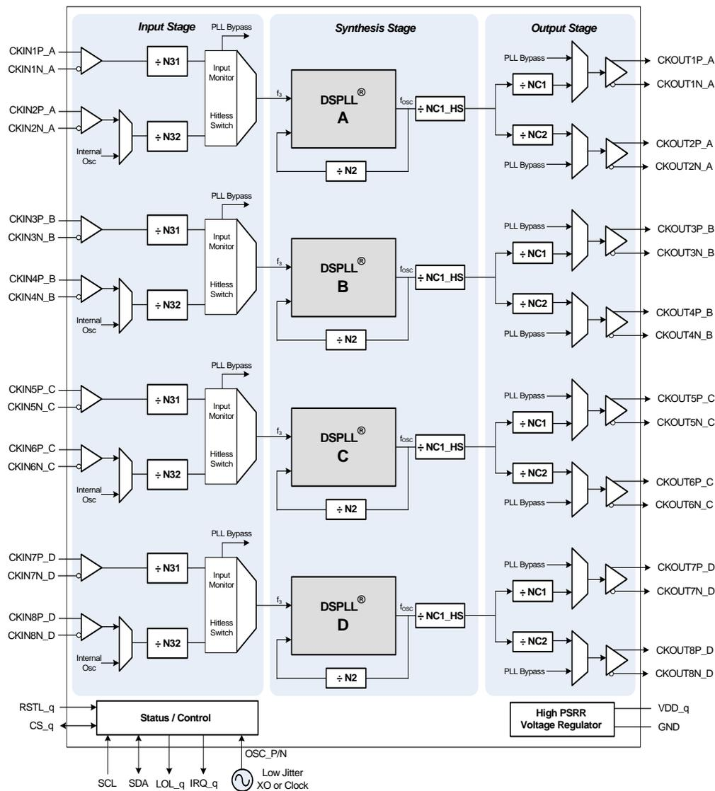
Figure 14. Si5374 Functional Block Diagram
