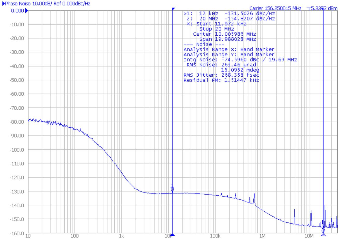
Figure 67. 19.44 MHz In; 156.25 MHz Out; Loop BW = 80 Hz
