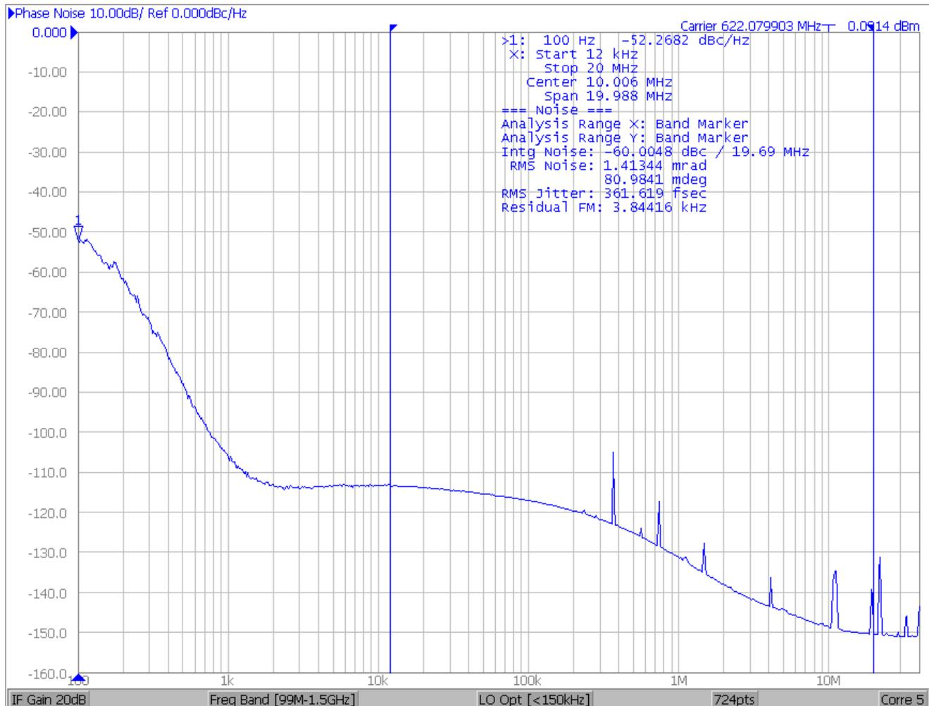
Figure 64. 622.08 MHz Output with a 40 MHz Crystal
