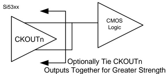
**Figure 42. Typical CMOS Output Circuit (Tie CKOUTn+ and CKOUTn- Together)**
