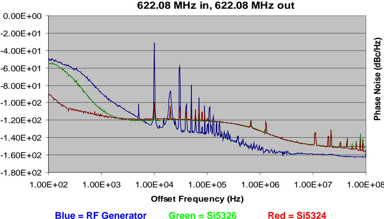
Figure 94. RF Generator, Si5326, Si5324 (10 kHz Jitter)
