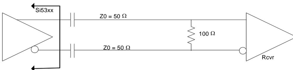
**Figure 40. Typical Output Circuit (Differential)**
