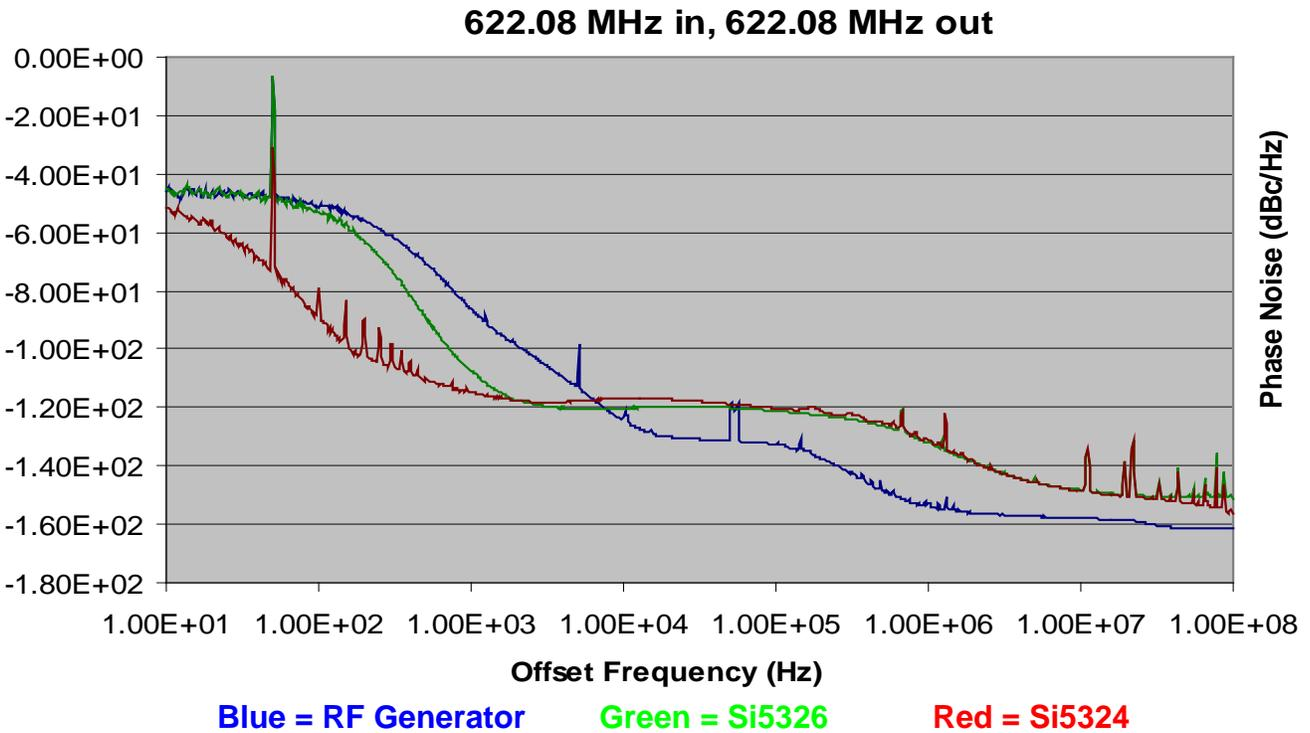
Figure 89. RF Generator, Si5326, Si5324 (50 Hz Jitter)
