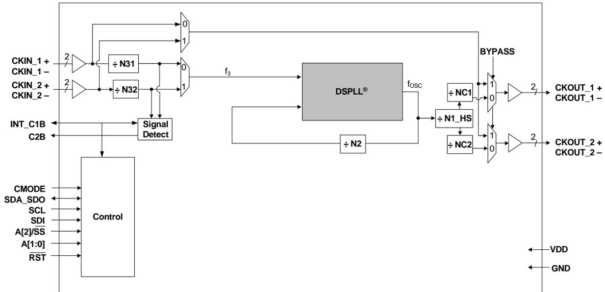
**Figure 6. Si5325 Low Jitter Clock Multiplier Block Diagram**
