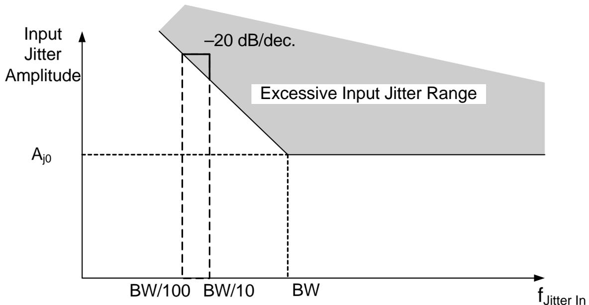
**Figure 20. Jitter Tolerance Mask/Template**
