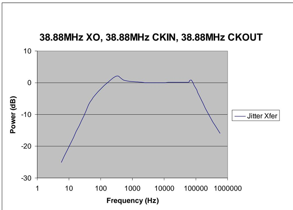
Figure 57. Typical Reference Jitter Transfer Function
