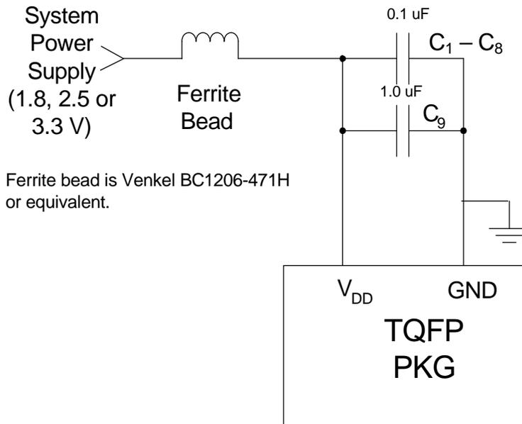
Figure 55. Typical Power Supply Bypass Network (TQFP Package)
