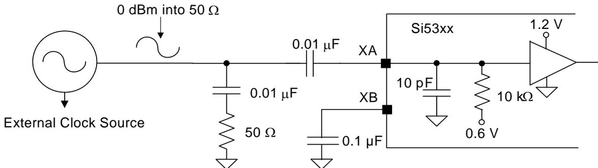
**Figure 50. Sinewave External Clock Circuit**
