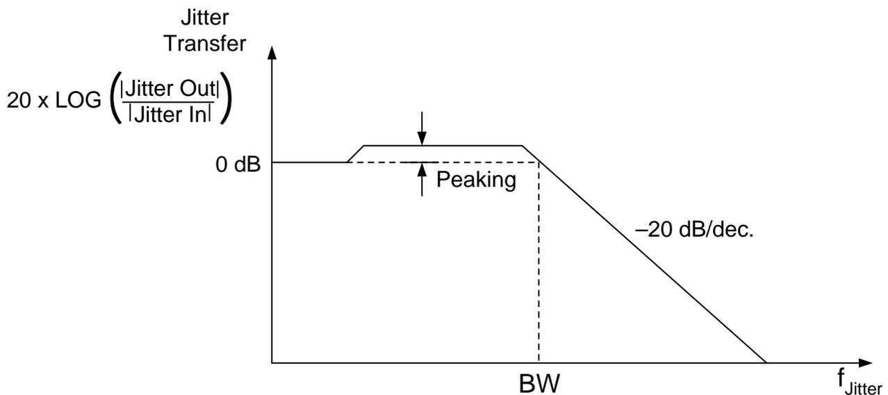
Figure 19. PLL Jitter Transfer Mask/Template
