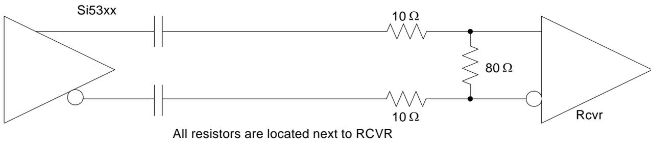
**Figure 41. Differential Output Example Requiring Attenuation**
