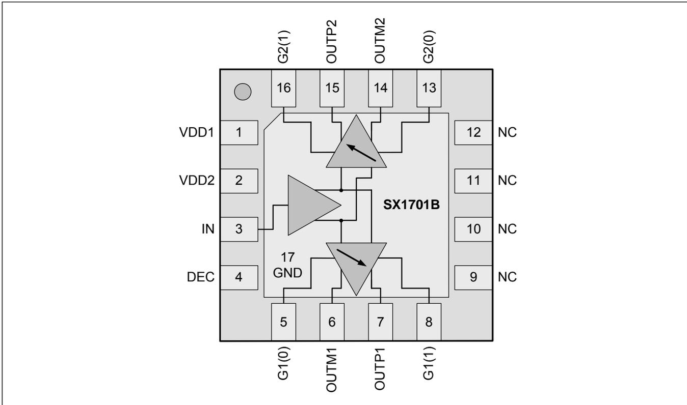
Figure 1. Simplified block diagram of the SX1701B.
