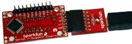
Finally, if you'll be mounting the display, any 4-40 screw should be able to find its way through those stand-off holes.
