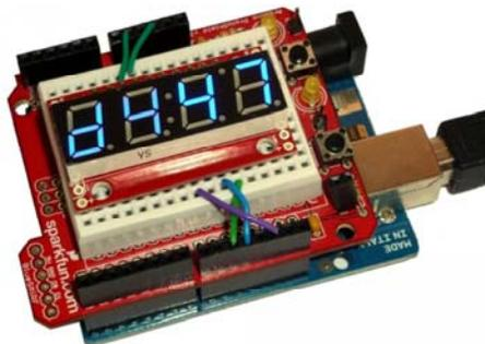
Of course, you could solder stranded or solid-core wires into the pins you need. This is useful if you plan on mounting the display in an enclosure.
