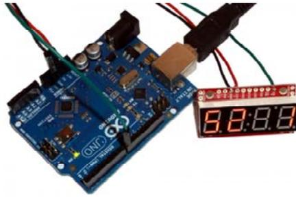
If you intend to ever reprogram the display using an FTDI Basic, you might find it useful to solder some right-angle male headers into the serial programming header. This can be a bit tricky, as the display gets in the way. I solder my right-anglers on the curved side.
