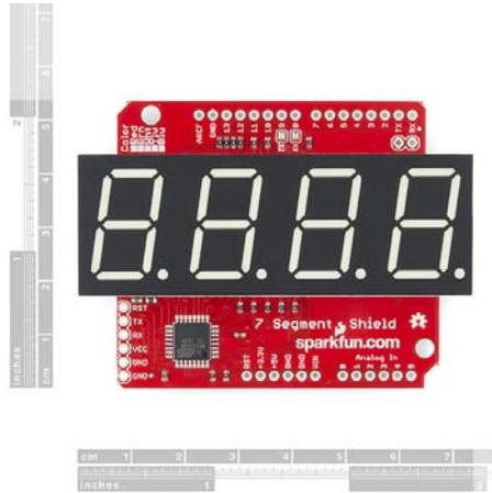
So what about I2C? Well while I2C can't be disabled in the same manner, it shouldn't conflict with another I2C device on the same bus unless they share the same address. In this case, you can reprogram the shield's firmware with a different I2C address. The shield's I2C address is 0x71 by default.
