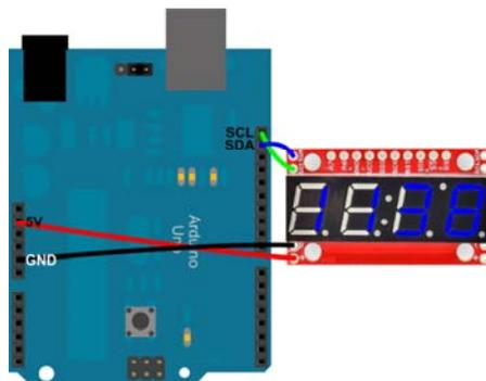
There's not any give in this pin configuration; you'll have to use the hardware I<sup>2</sup>C pins. Older Arduinos may not have the devoted SDA and SCL pins. They should still be there, on pins A4 and A5 respectively.
