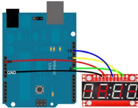
The SDI and SCK pins must remain where they are on the Arduino - those are the hardware SPI pins. The SS pin could be moved to any digital pin, as long as it's changed in the code.
