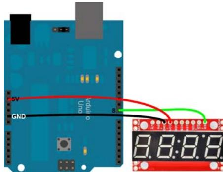
Really, you can use any digital pin to serve as the Arduino's software TX pin. Just make sure you change it in the code. Speaking of the code copy/past this, or you can download it from here:
