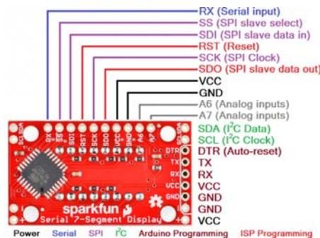
It'll be your choice to decide which of the three serial interfaces you'd like to use to connect to the display. Using a basic serial input, you'll only need to connect to the RX pin. I<sup>2</sup>C requires two pins, and SPI requires three.
