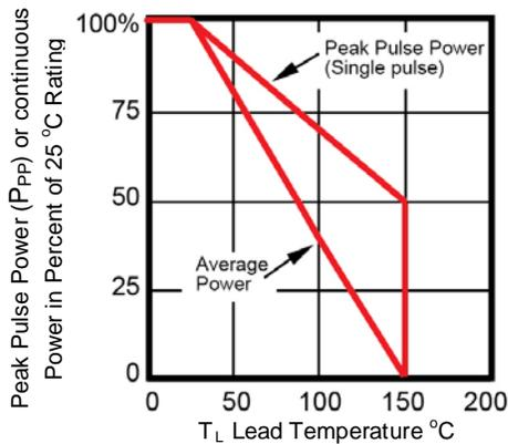
FIGURE 3 – Derating Curve
