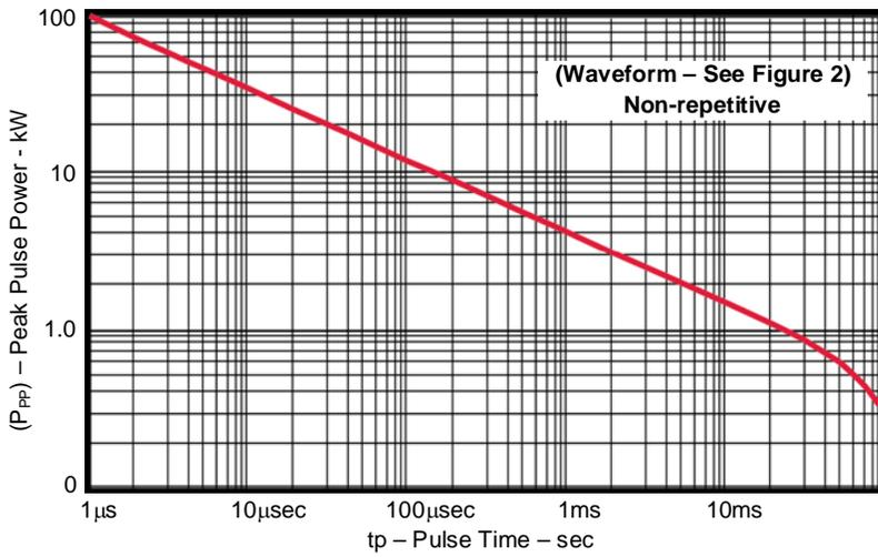
FIGURE 1 – Peak Pulse Power vs. Pulse Time
