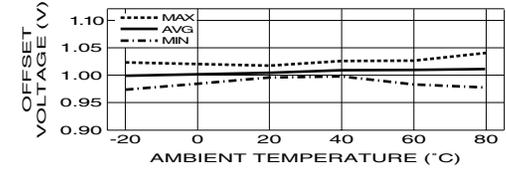
Output Voltage vs Temperature
