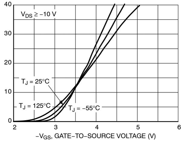
Figure 2. Transfer Characteristics
