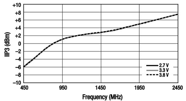
Figure 6. IIP3 Over Supply Voltage and Frequency
