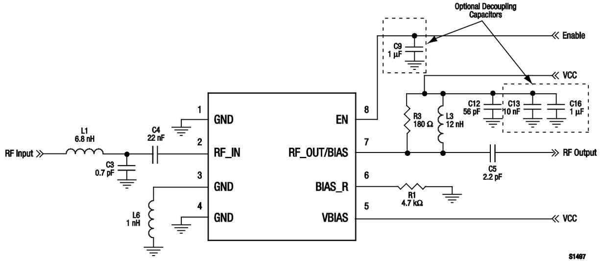
Figure 9. SKY65047-360LF Evaluation Board Schematic (915 MHz)
