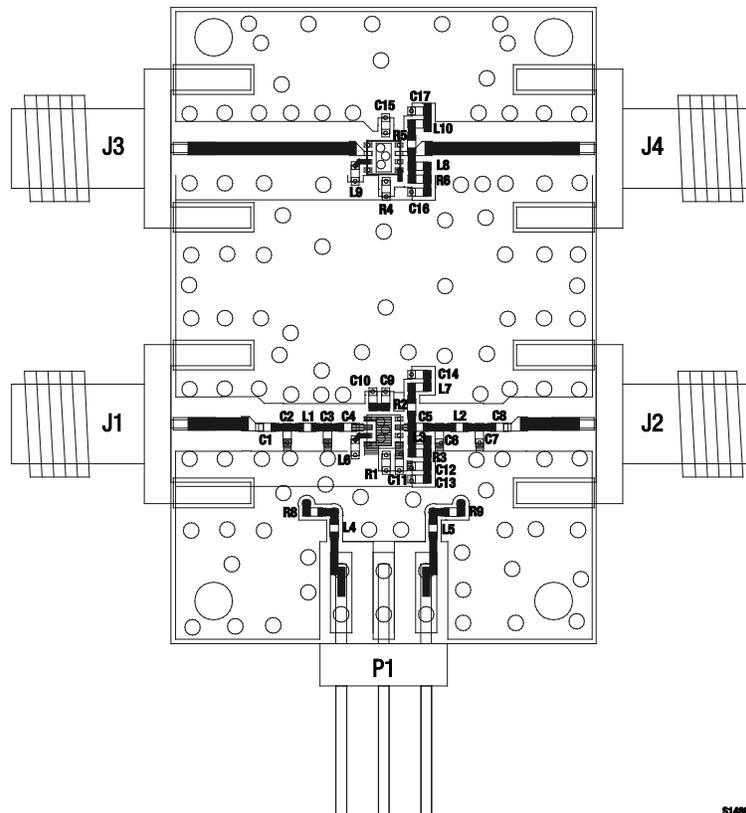
Figure 10. SKY65047-360LF Evaluation Board Assembly Diagram (915 MHz)
