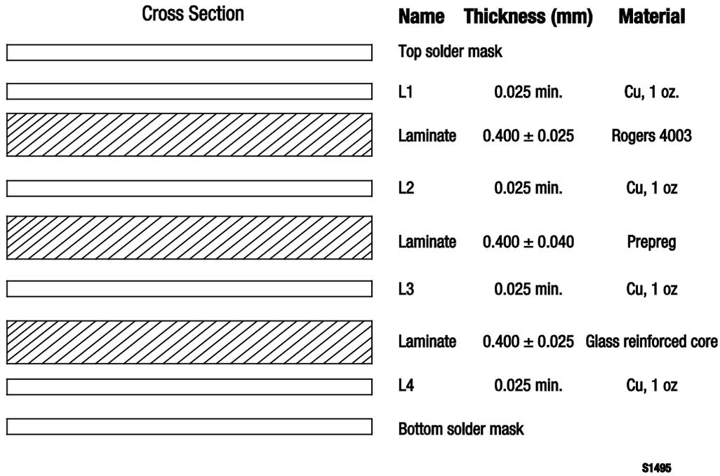
Figure 18. Layer Detail Physical Characteristics
