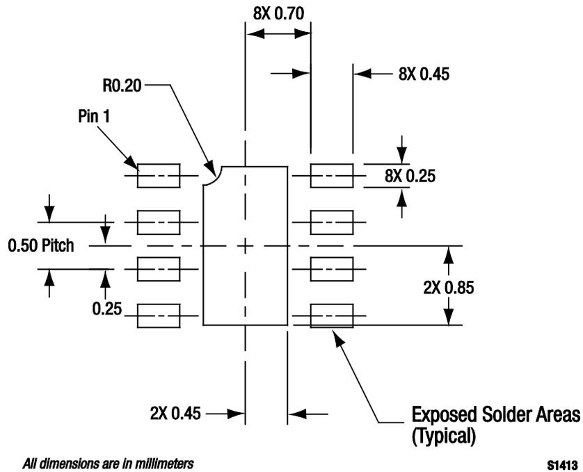
Figure 19. SKY65047-360LF PCB Layout Footprint (Top View)
