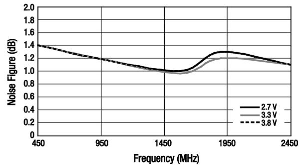
Figure 8. Noise Figure Over Supply Voltage and Frequency
