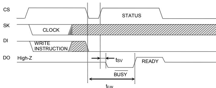
Figure 48. READY/ $\overline{\text{BUSY}}$  STATUS output timing chart
