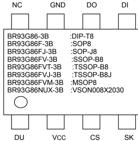
Figure 3. Pin Configuration
