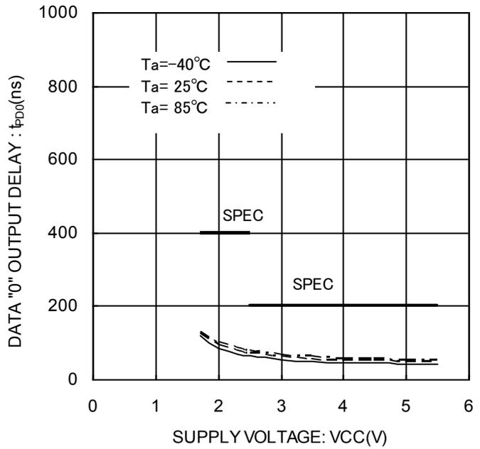
Figure 29. Data "0" output delay  $t_{PO0}$
