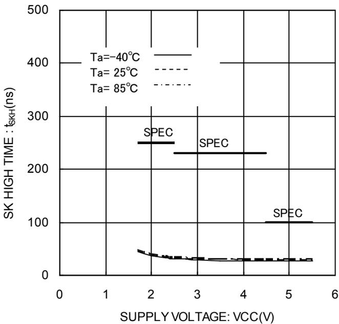
Figure 22. SK high time t<sub>SKH</sub>
