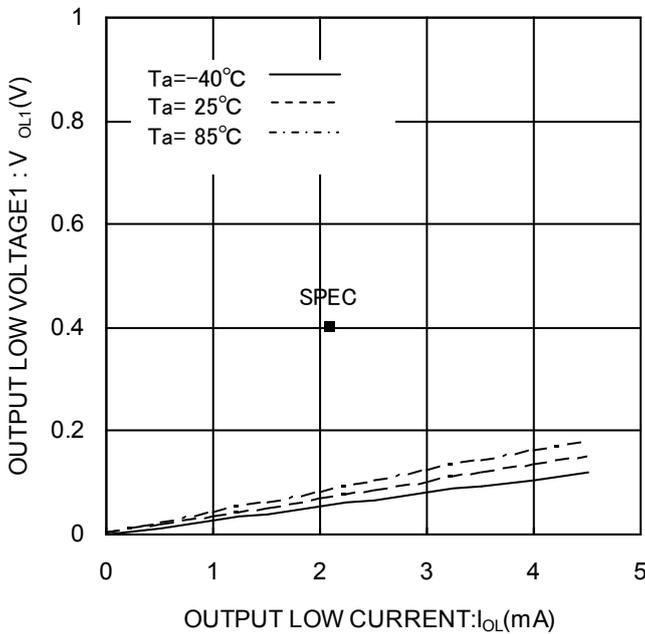
Figure 6. Output low voltage1  $V_{OL1}$ ( $V_{CC}=2.7\text{V}$ )
