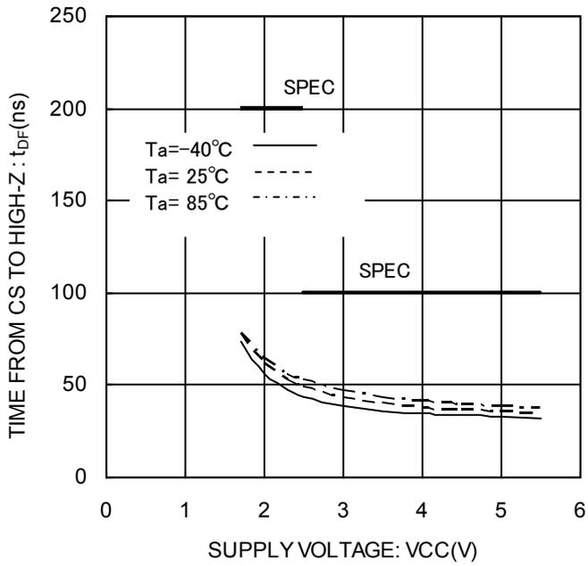
Figure 32. Time from CS to High-Z  $t_{Dr}$
