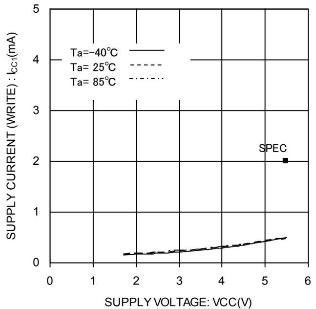
Figure 15. Supply current (WRITE)
