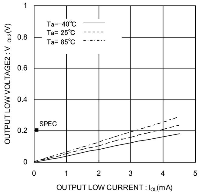
Figure 7. Output low voltage2  $V_{OL2}$ ( $V_{CC}=1.7\text{V}$ )
