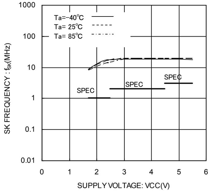
Figure 21. SK frequency f<sub>SK</sub>
