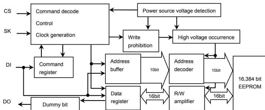
Figure 2. Block diagram
