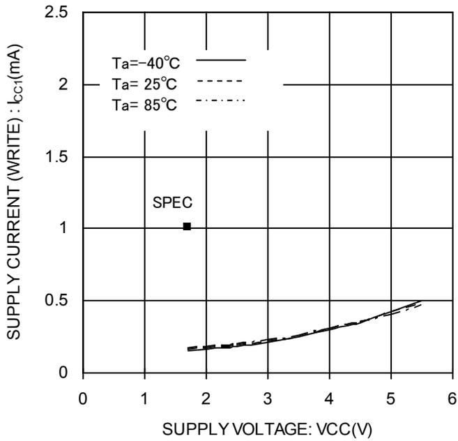
Figure 14. Supply current (WRITE)
