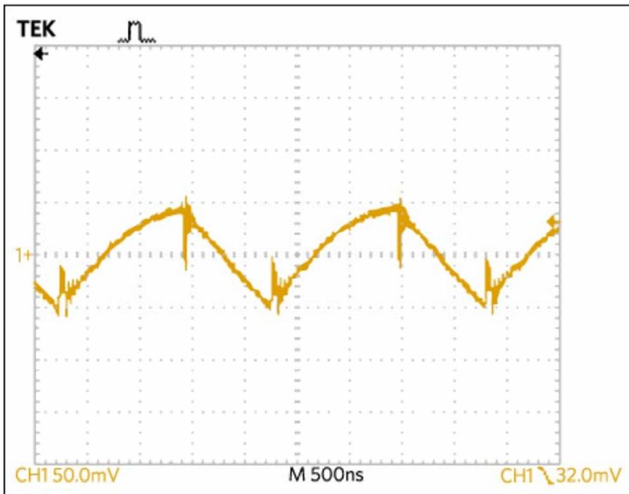
Figure 3. Output ripple at 800mA load, 12V<sub>out</sub>.
