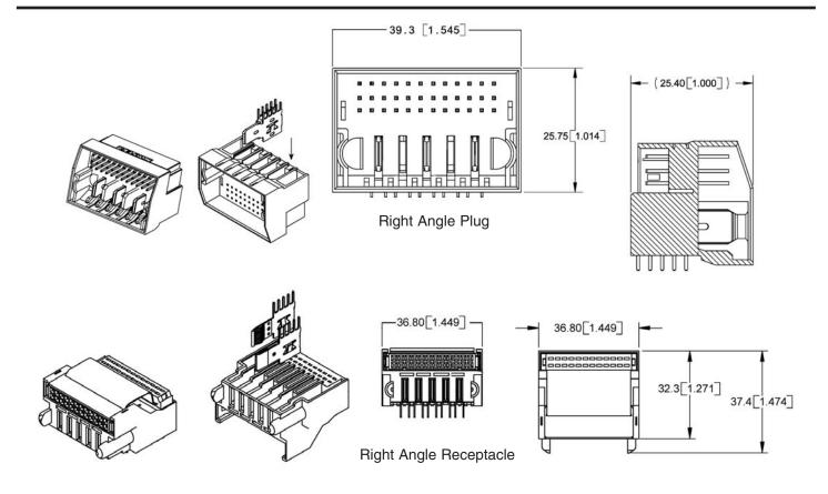
**Dual Blade Contact**Provides two 15 Amp contacts in the space of one 30 Amp contact
