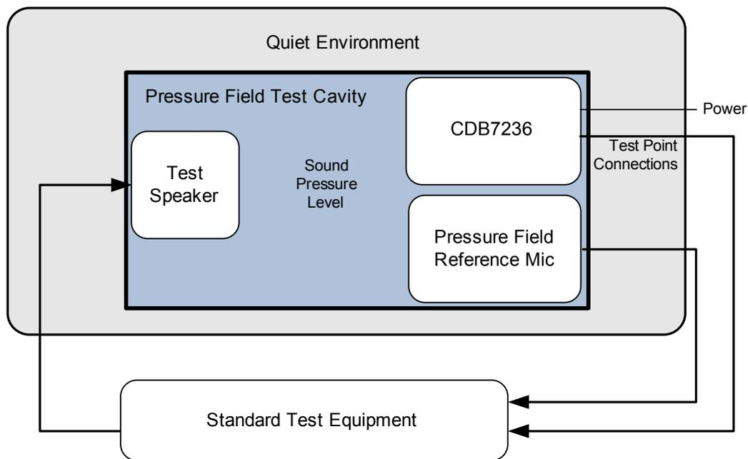
**Figure 2-1. Pressure field test setup with CDB7236**
