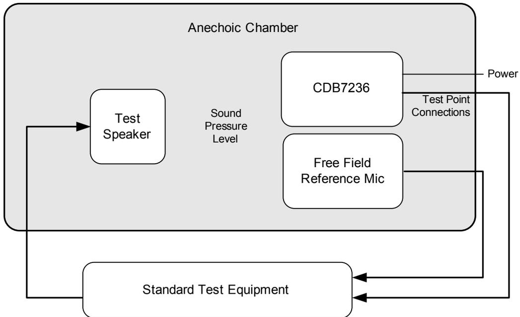
**Figure 2-2. Free field test setup with CDB7236**
