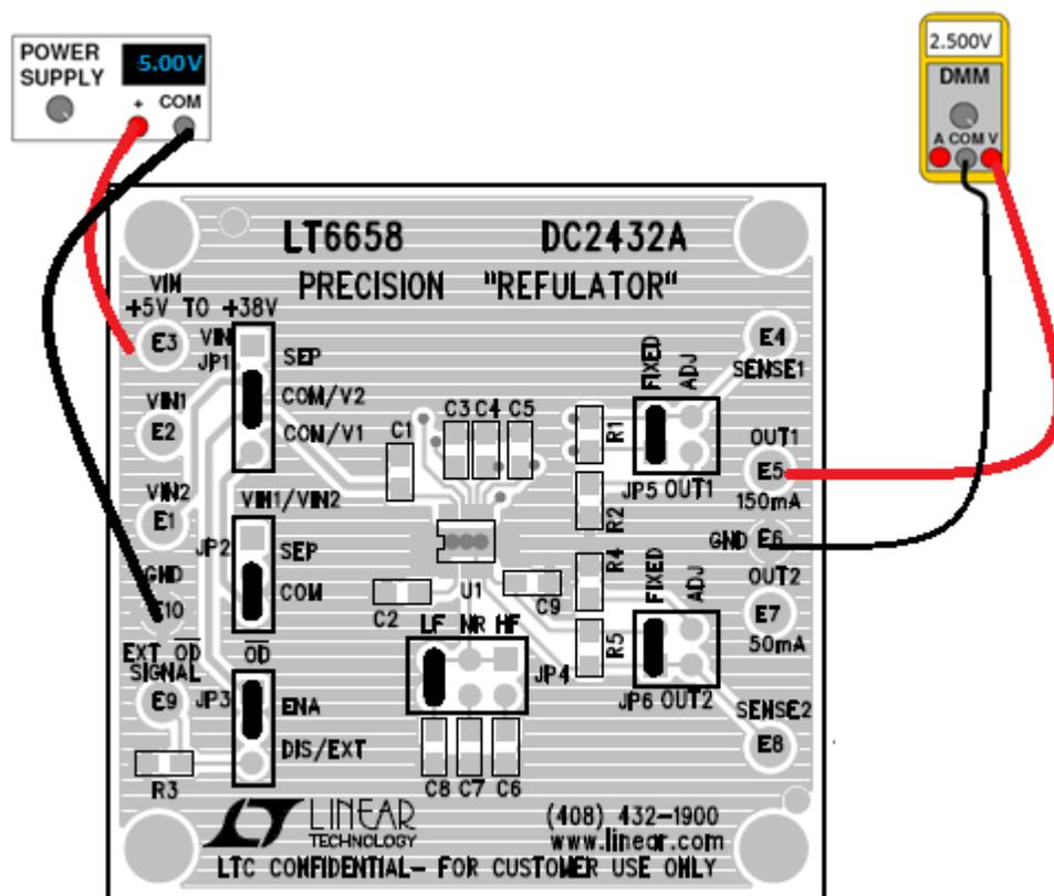
Figure 1: Test Setup
