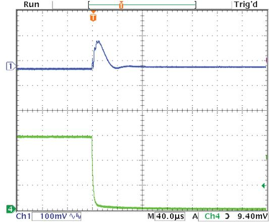
Step Load Transient Response (Vin=7.5V, Vout=5V, Cload=10x10µF X5R 0805 ceramic, plus 1x470µF, 7mΩ POSCAP, total 570µF, Iout=0A to 3A) Top trace=Vout, Bottom trace=Iout
