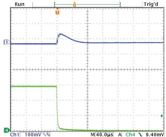
Step Load Transient Response (Vin=12V, Vout=1.8V, Cload=10x10µF X5R 0805 ceramic, plus 1x470µF, 7mΩ POSCAP, total 570µF, Iout=0A to 3A) Top trace=Vout, Bottom trace=Iout
