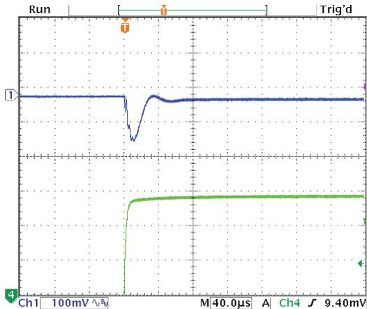
Step Load Transient Response (Vin=12V, Vout=3.3V, Cload=12x10µF
