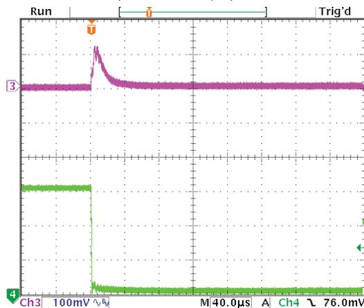
Step Load Transient Response (Vin=4.5V, Vout=1.8V, Cload=5x10µF
