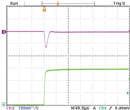
Step Load Transient Response (Vin=4.5V, Vout=1.8V, Cload=5x10µF
