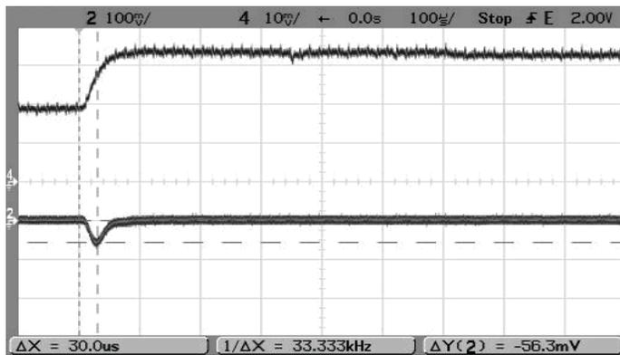
Step Load Transient Response (Vin=12V, Vout=2.5V, Cload=0, Iout=3A to 1.5A)
