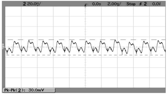
Step Load Transient Response (Vin=12V, Vout=2.5V, Cload=0, Iout=1.5A to 3A)
