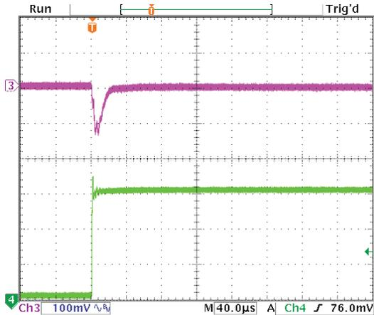
Step Load Transient Response (Vin=12V, Vout=3.3V, Cload=5x10µF
