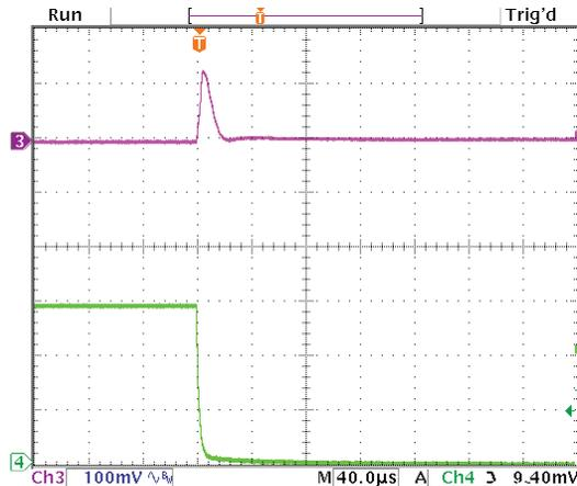
Step Load Transient Response (Vin=12V, Vout=1.8V, Cload=12x10µF
