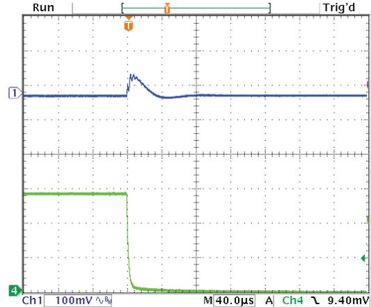
Step Load Transient Response (Vin=12V, Vout=5V, Cload=10x10µF X5R 0805 ceramic, plus 1x470µF, 7mΩ POSCAP, total 570µF, Iout=0A to 3A) Top trace=Vout, Bottom trace=Iout
