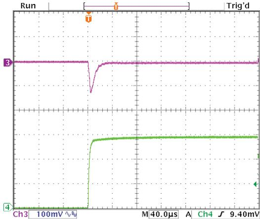
Step Load Transient Response (Vin=5.5V, Vout=3.3V, Cload=5x10µF
