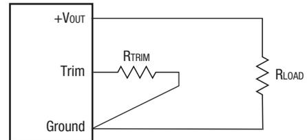
$$R_{TRIM} (k\Omega) = \frac{1.182}{V_{OUT} - 0.591}$$
