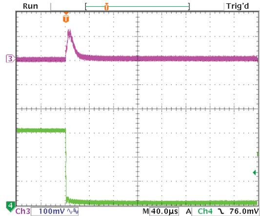
Step Load Transient Response (Vin=5.5V, Vout=3.3V, Cload=5x10µF
