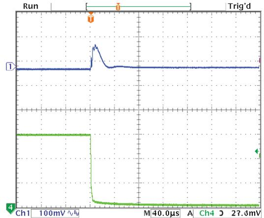
Step Load Transient Response (Vin=4.5V, Vout=1.8V, Cload=10x10µF X5R 0805 ceramic, plus 1x470µF, 7mΩ POSCAP, total 570µF, Iout=0A to 3A) Top trace=Vout, Bottom trace=Iout
