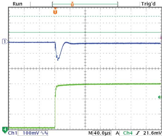
Step Load Transient Response (Vin=4.5V, Vout=1.8V, Cload=12x10µF X5R 0805 ceramic, total 120µF, Iout=3A to 0A) Top trace=Vout, Bottom trace=Iout
