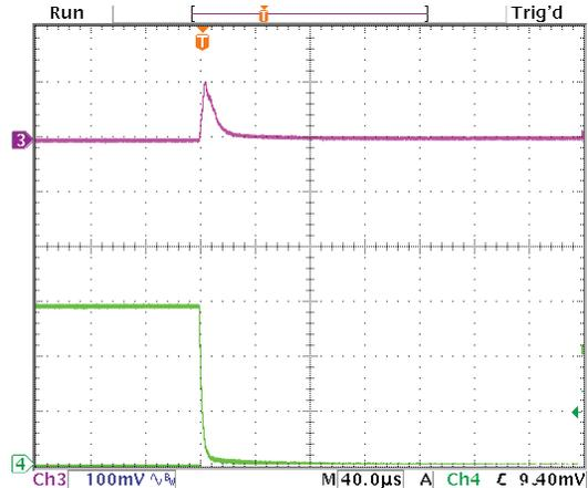
Step Load Transient Response (Vin=12V, Vout=5V, Cload=12x10µF X5R 0805 ceramic, total 120µF, Iout=0A to 3A) Top trace=Vout, Bottom trace=Iout
