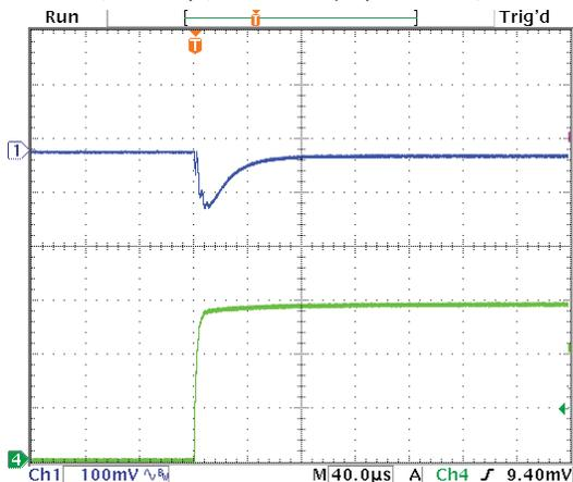
Step Load Transient Response (Vin=12V, Vout=1.8V, Cload=12x10µF
