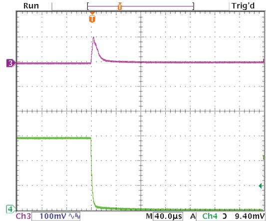
Step Load Transient Response (Vin=12V, Vout=3.3V, Cload=12x10µF
