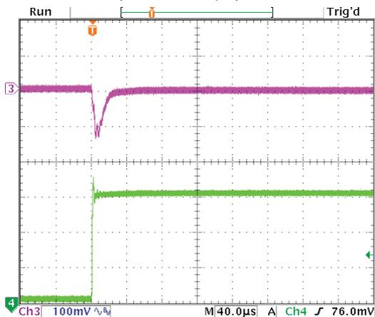
Step Load Transient Response (Vin=12V, Vout=1.8V, Cload=5x10µF
