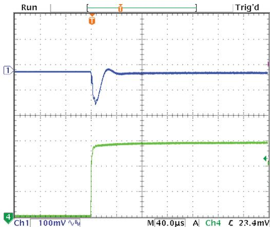
Step Load Transient Response (Vin=5.5V, Vout=3.3V, Cload=12x10µF X5R 0805 ceramic, total 120µF, Iout=3A to 0A) Top trace=Vout, Bottom trace=Iout
