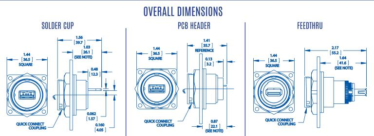
Note: Dimension does not include gasket compression. Dimensions in inches [mm]. Quick connect option shown. See drawings from Conxall.com for detailed dimensions
