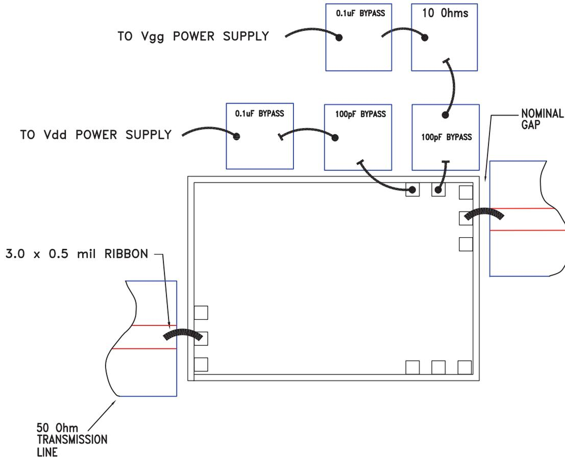
Note 1: Bypass caps should be 100 pF (approximately) ceramic (single-layer) placed no farther than 30 mils from the amplifier.
