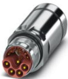
Coupling connector, straight long, shielded: yes, Screw locking, M23, Number of positions: 4+4+4+PE / 3+N +PE, Type of contact: Pin, Crimp connection, Cable diameter: 9 mm ... 12 mm
