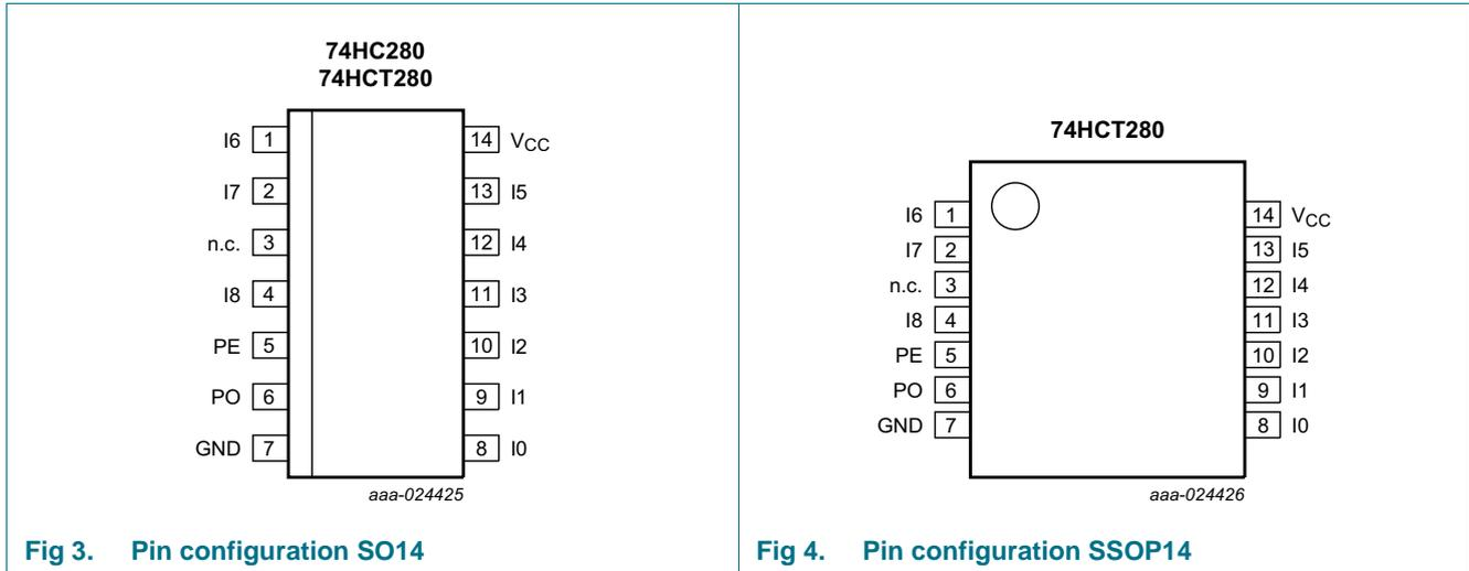
Fig 3. Pin configuration SO14
