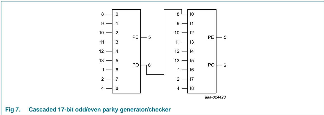
**Fig 7. Cascaded 17-bit odd/even parity generator/checker**
