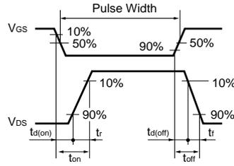
Fig.1-2 Switching Waveforms
