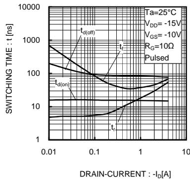
Fig.11 Switching Characteristics
