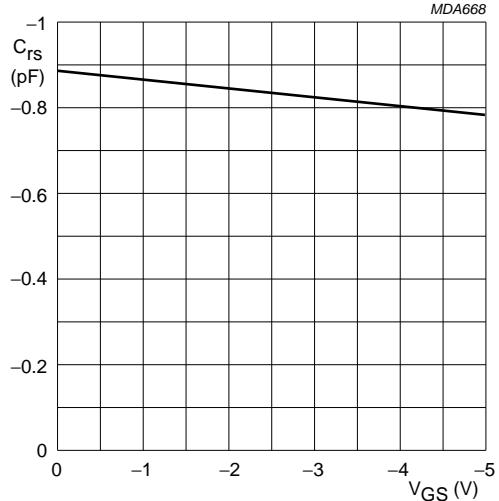
$V_{DS} = 10$  V;  $f = 1$  MHz;  $T_{amb} = 25$  °C.
