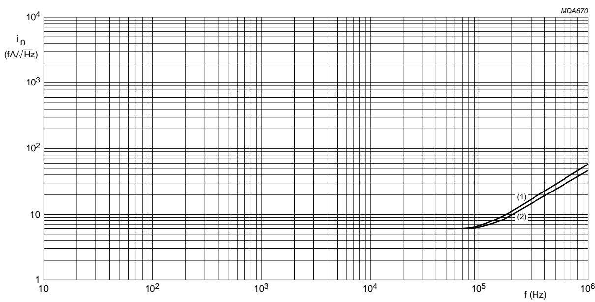
$V_{DS} = 10 \text{ V}; T_{amb} = 25^\circ\text{C}.$ (1) BFR31;  $I_D = 1 \text{ mA}$ .(2) BFR30;  $I_D = 4 \text{ mA}$ .
