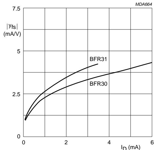
$V_{DS} = 10$  V;  $f = 1$  kHz;  $T_{amb} = 25$  °C.
