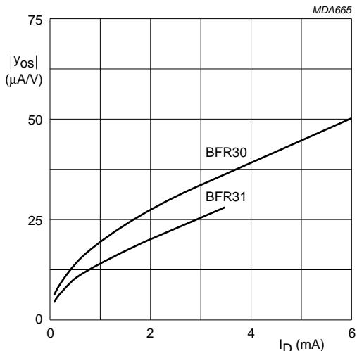
$V_{DS} = 10$  V;  $f = 1$  kHz;  $T_{amb} = 25$  °C.
