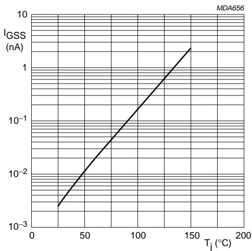
$V_{GS} = -10 \text{ V}; V_{DS} = 0$ .
