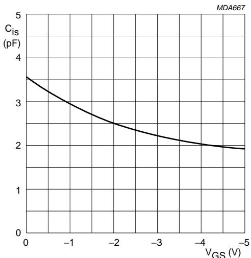
$V_{DS} = 10$  V;  $f = 1$  MHz;  $T_{amb} = 25$  °C.
