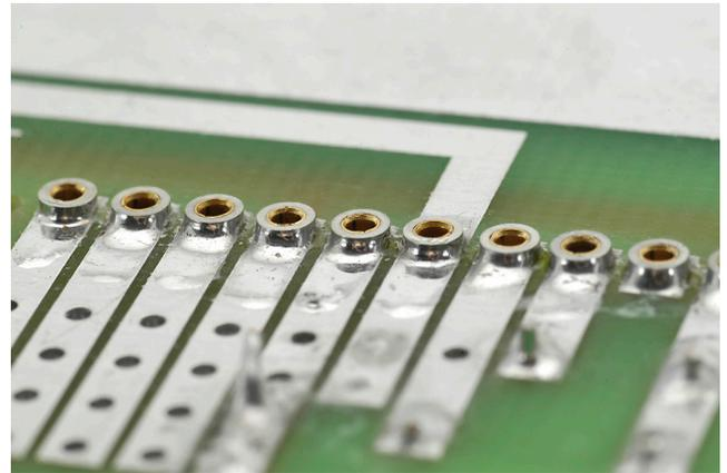
Part number MS11 consists of a carrier strip of 30 cage jacks. The strip can easily be cut to any desired number of cage jacks. These are mounted directly in a print circuit board. After soldering, the carrier is pulled off the cage jacks. Use a spacer between the PCB and the heatsink to avoid short circuits.
