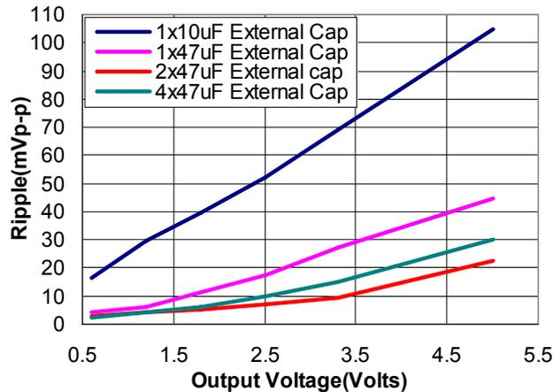
**Note:** Output ripple voltage for various output voltages with external 1x10  $\mu$ F, 1x47  $\mu$ F, 2x47  $\mu$ F or 4x47  $\mu$ F ceramic capacitors at the output (3A load). Input voltage is 12V.
