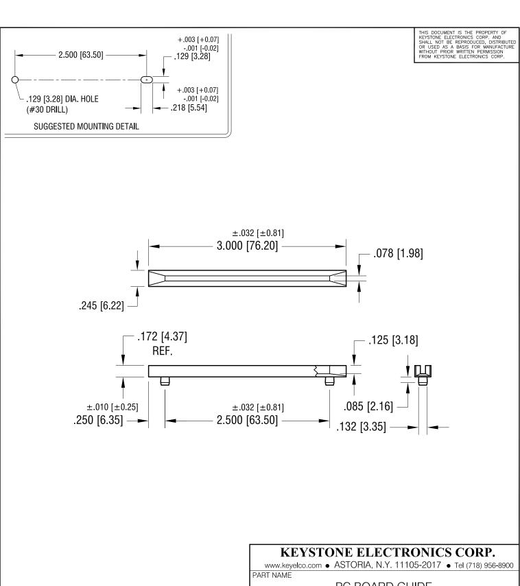
PC BOARD GUIDE MATERIAL NATURAL NYLON 6/6 UL 94V-2 DRN BY FINISH **BOONE** 3.7.00 APP'D SCALE LN 1X CHANGE AS PER ECN 15-138 11.23.15 Α TOLERANCES INCH [MM] CODE DWG NO.  $\pm .005 [\pm 0.13]$ DECIMAL 8621 C ANGULAR ± 1° DATE **DESCRIPTION** REV. UNLESS OTHERWISE SPECIFIED
