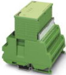
INTERBUS-ST analog input module, 2 inputs, 0 to 20 mA, 4 to 20 mA, 0 to 10 V, IP20 protection, consisting of: Terminal part with screw connection and module electronics,
