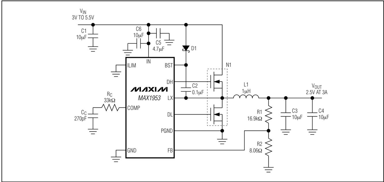
Figure 1. Typical Application Circuit for the MAX1953
