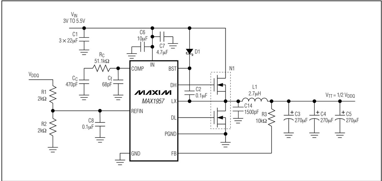
Figure 3. Typical Application Circuit for the MAX1957
