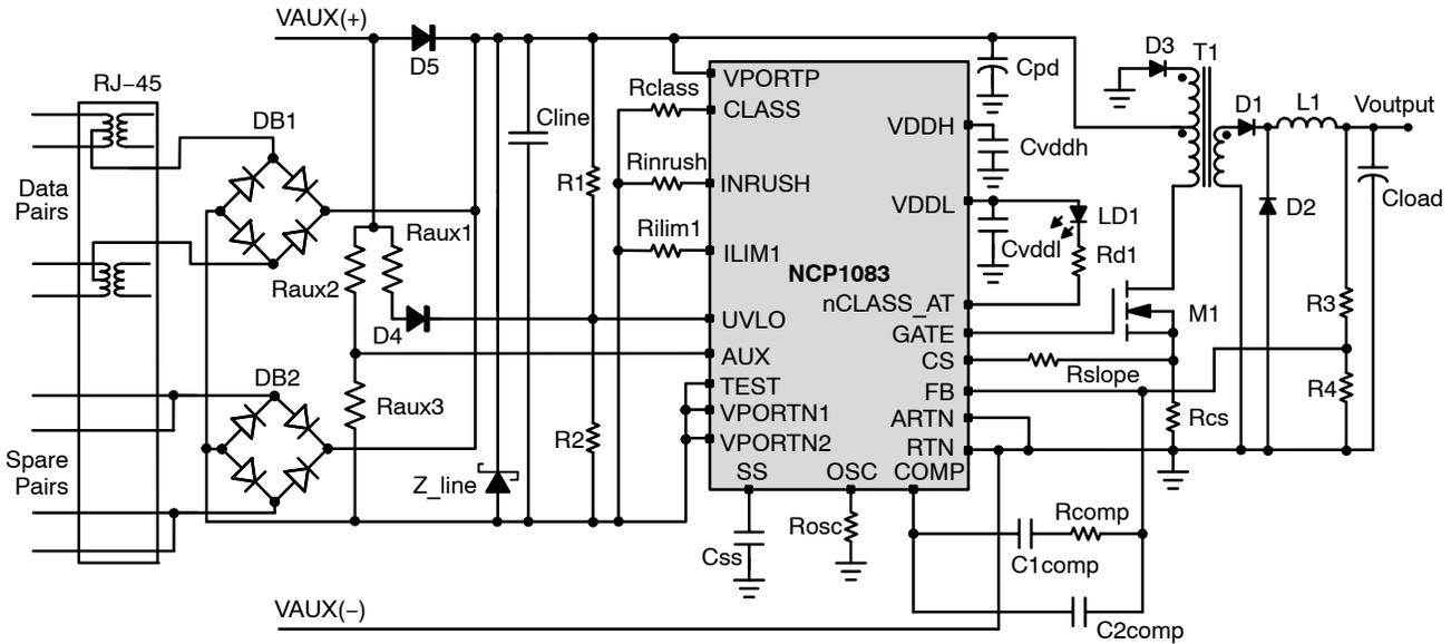
**Figure 5. Non-Isolated Forward Converter with Rear Auxiliary Supply**
