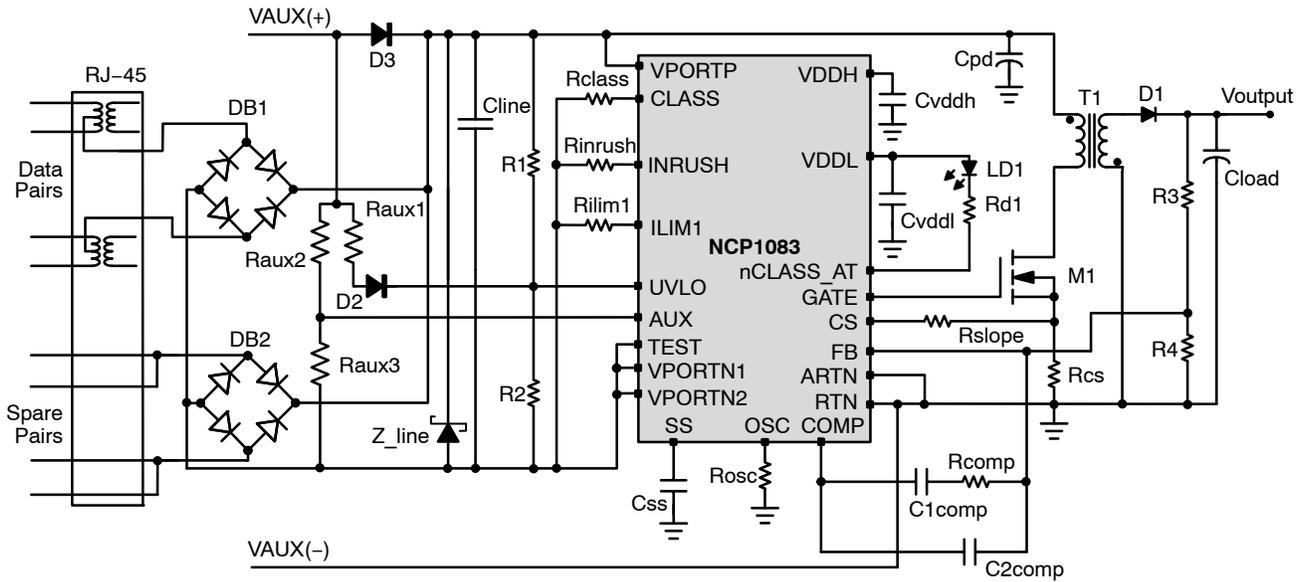
**Figure 3. Non-Isolated Fly-back Converter with Rear Auxiliary Supply**
