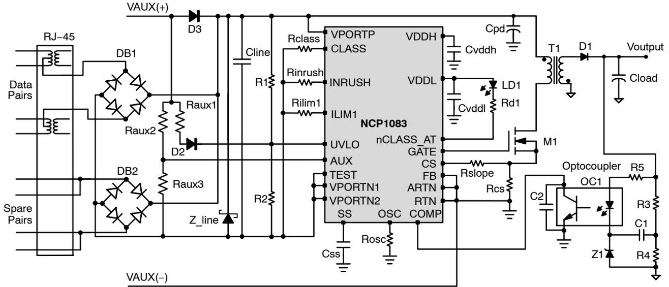
**Figure 2. Isolated Fly-back Converter with Rear Auxiliary Supply**
