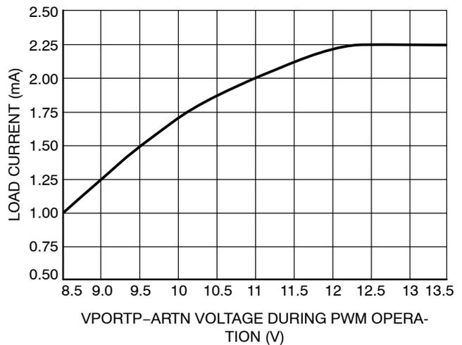
Figure 7. (I<sub>vddh\_load</sub>+I<sub>vddl\_load</sub>)<sub>max</sub> with Auxiliary Supply Operation
