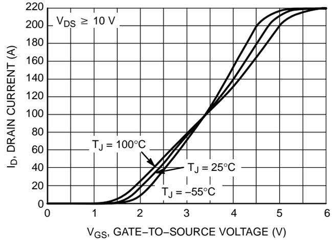
Figure 2. Transfer Characteristics
