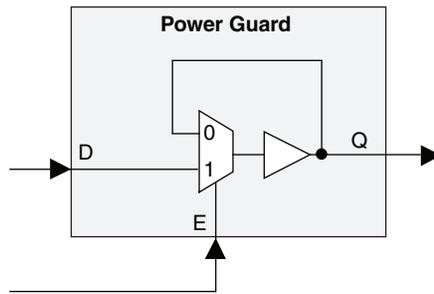
All the I/O pins in a block share a common Power Guard Enable signal. For a block of I/Os, this signal is called a Block Input Enable (BIE) signal. BIE can be internally generated using MC logic, or could come from external sources using one of the user I/O or input pins.
