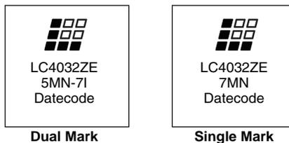
**Figure 20. Mark Format for 64 ucBGA and 132 ucBGA Packages**
