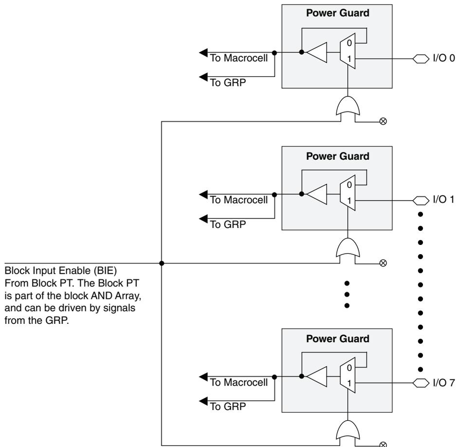
The number of BIE inputs, thus the number of Power Guard “Blocks” that can exist in a device, depends on the device size. Table 8 shows the number of BIE signals available in the ispMACH 4000ZE family. The number of I/Os available in each block is shown in the Ordering Information section of this data sheet.
