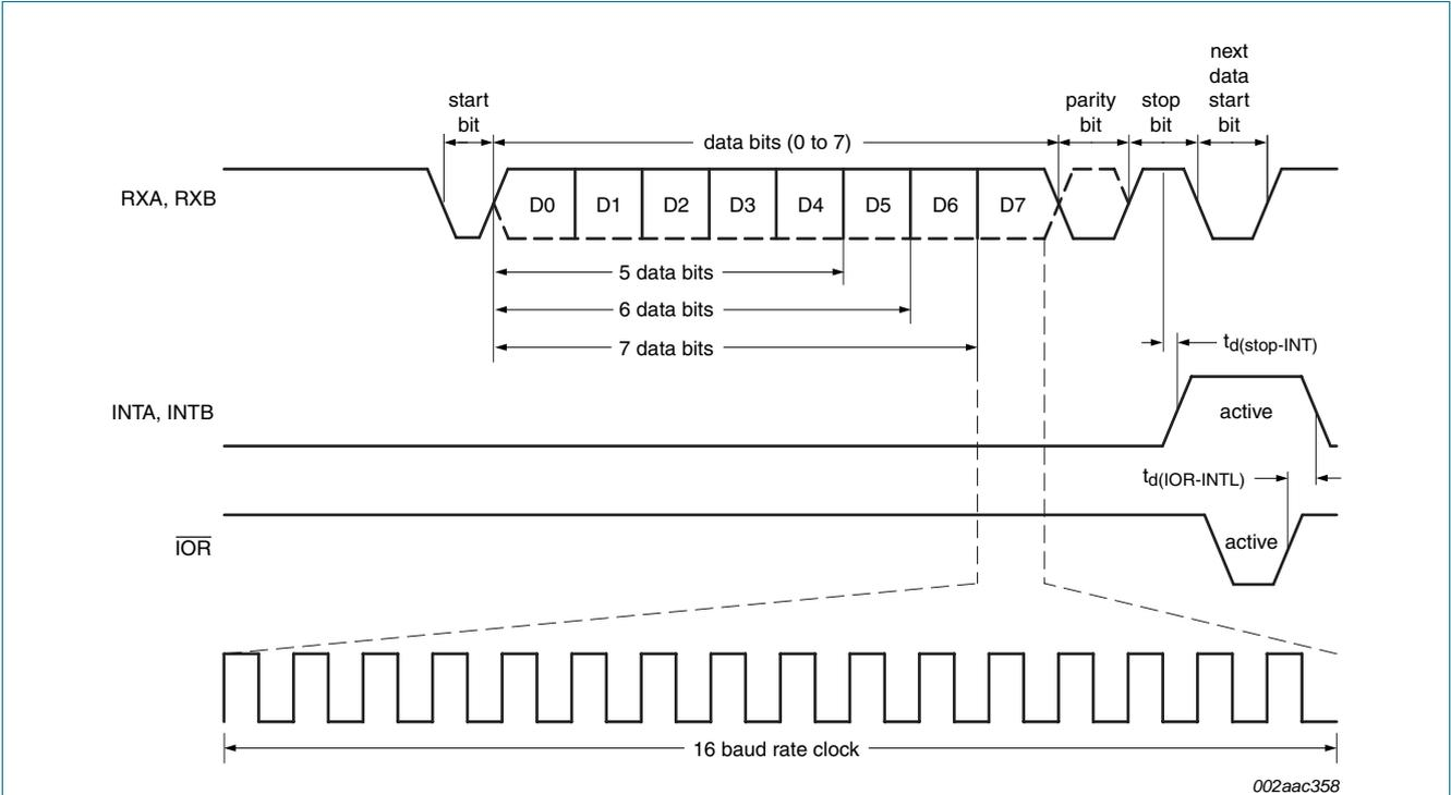
Fig 14. Receive timing
