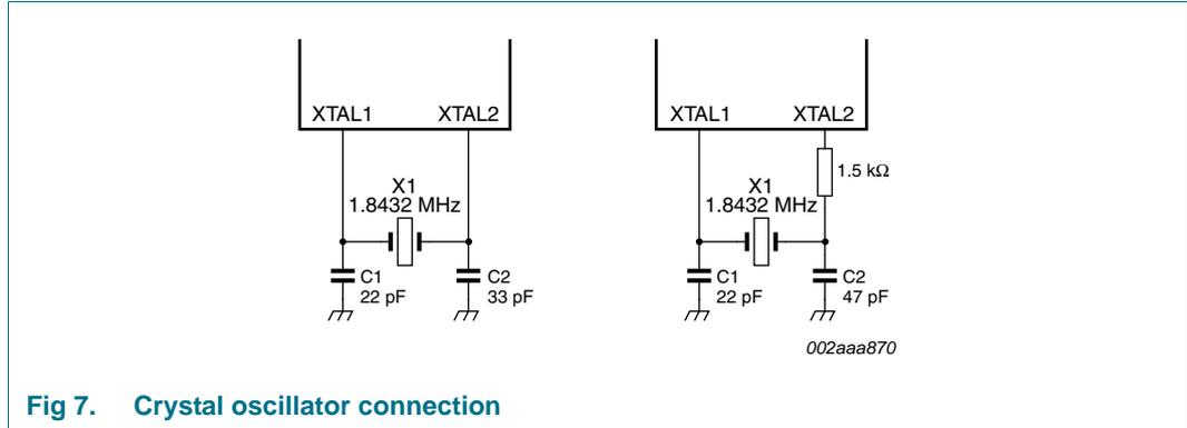
Fig 7. Crystal oscillator connection
