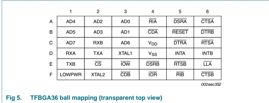
Fig 5. TFBGA36 ball mapping (transparent top view)
