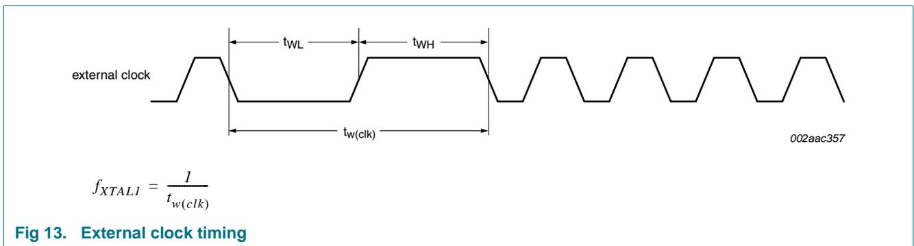
Fig 13. External clock timing
