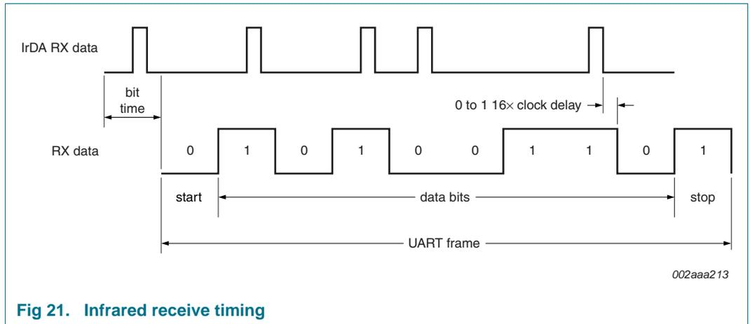
Fig 21. Infrared receive timing
