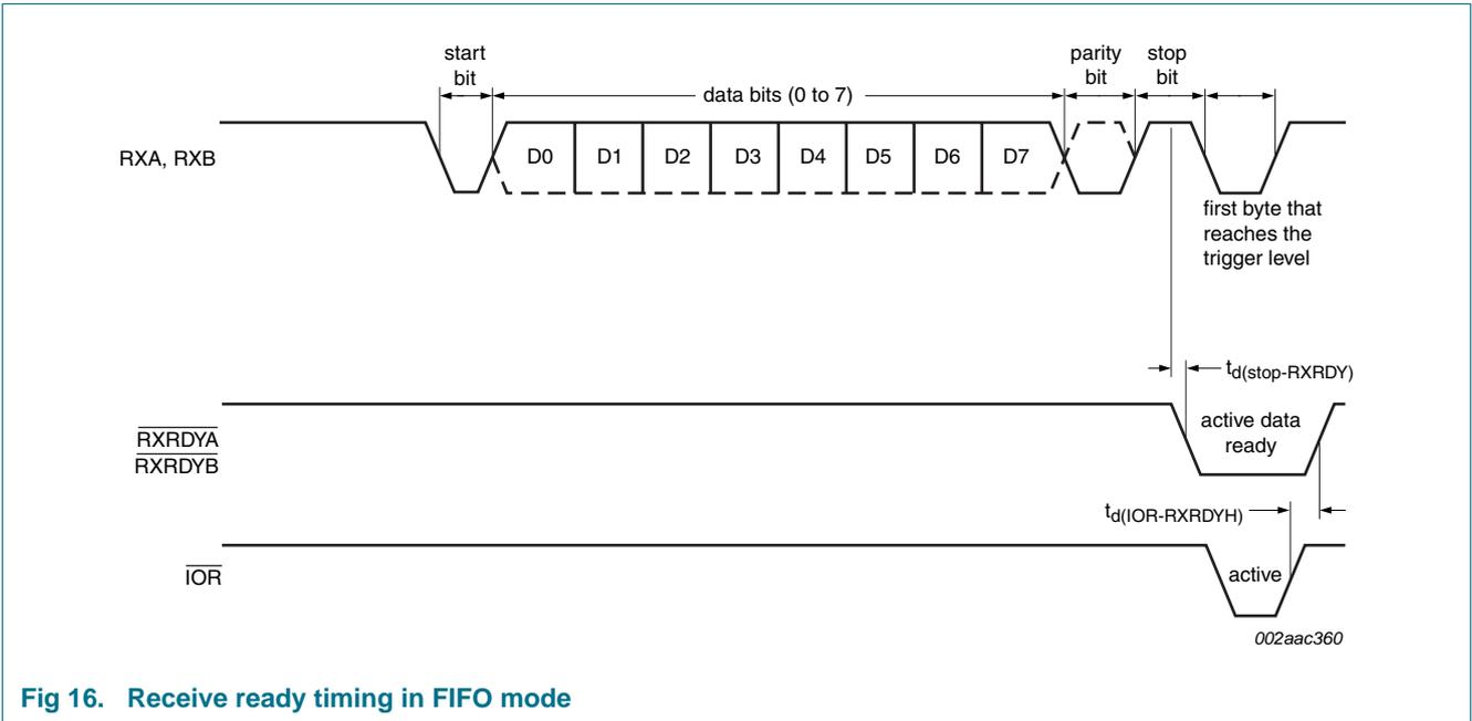
Fig 16. Receive ready timing in FIFO mode
