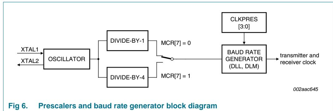
Fig 6. Prescalers and baud rate generator block diagram
