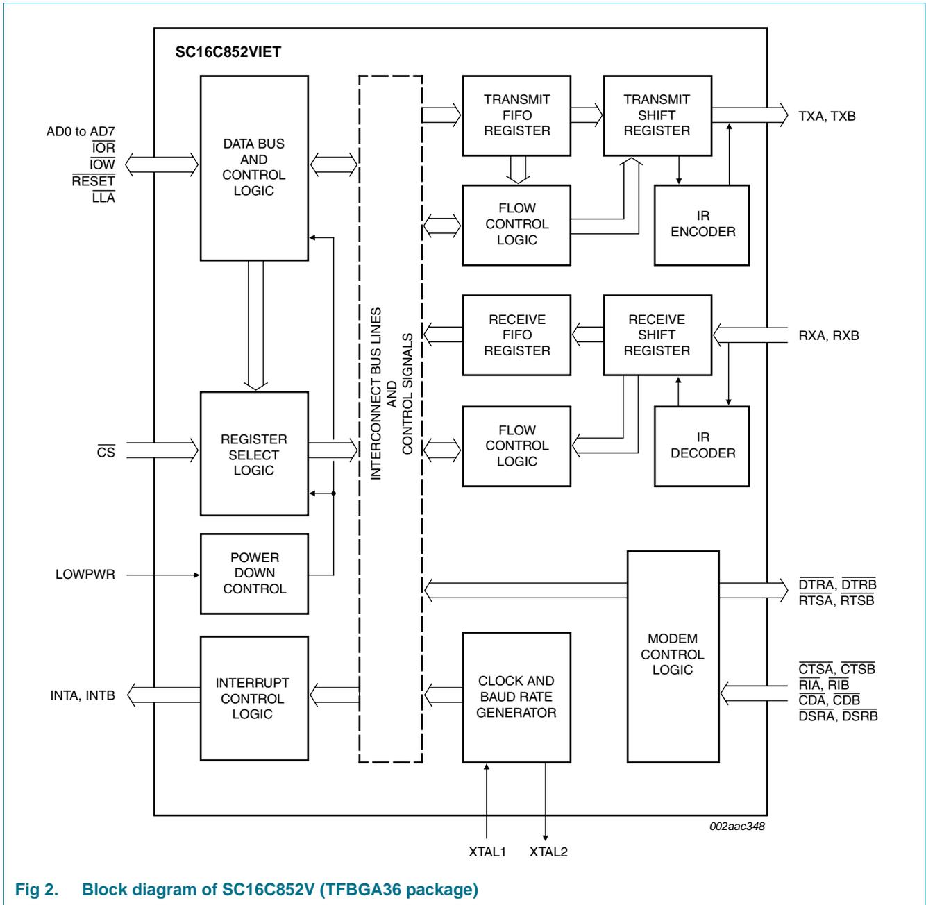
Fig 2. Block diagram of SC16C852V (TFBGA36 package)
