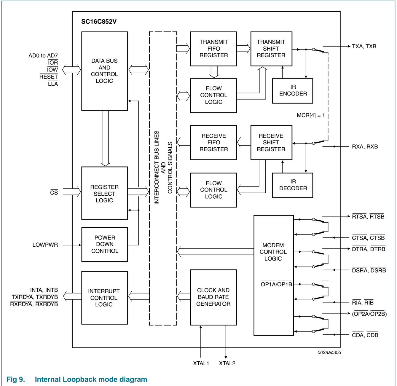
Fig 9. Internal Loopback mode diagram
