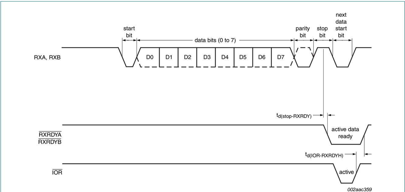
Fig 15. Receive ready timing in non-FIFO mode
