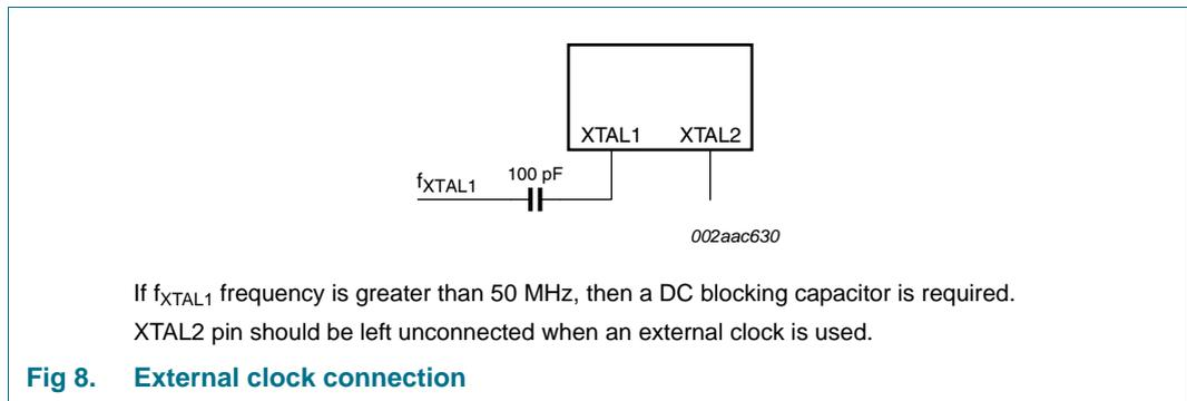
Fig 8. External clock connection
