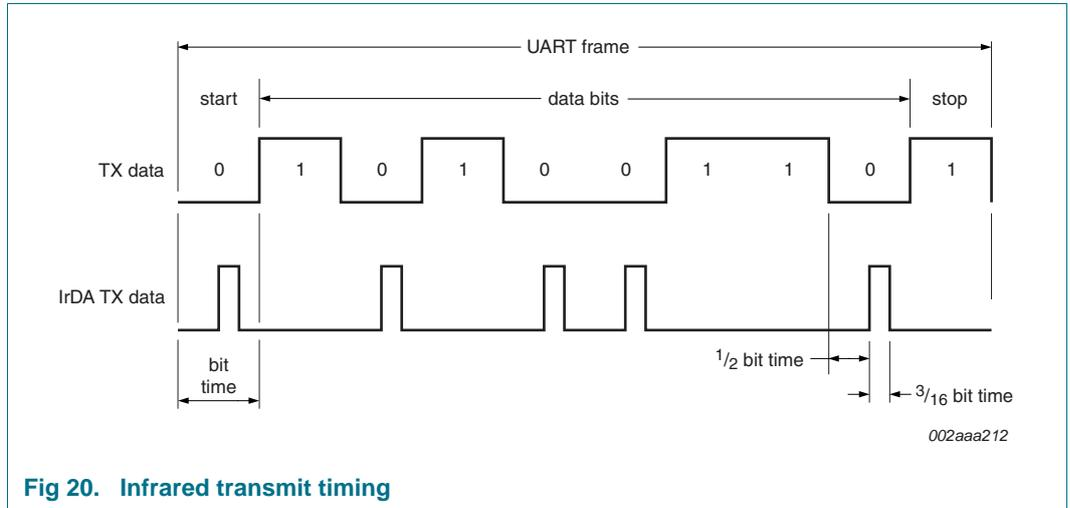
Fig 20. Infrared transmit timing
