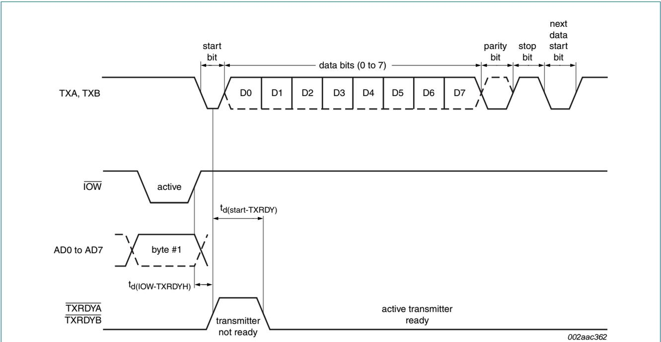
Fig 18. Transmit ready timing in non-FIFO mode
