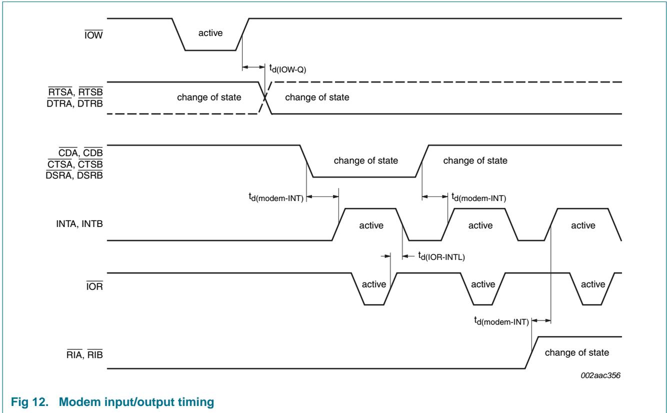
Fig 12. Modem input/output timing
