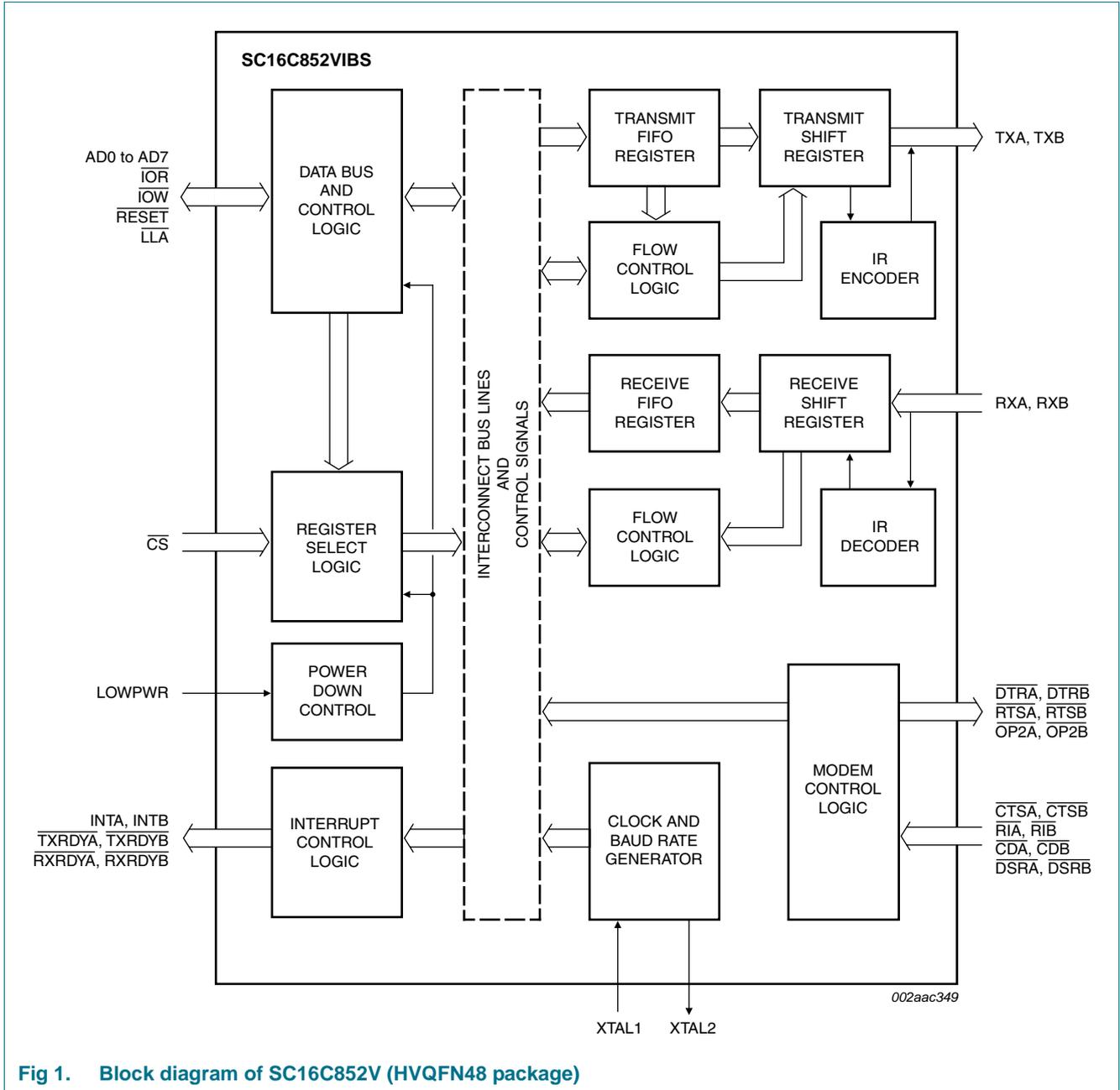
Fig 1. Block diagram of SC16C852V (HVQFN48 package)
