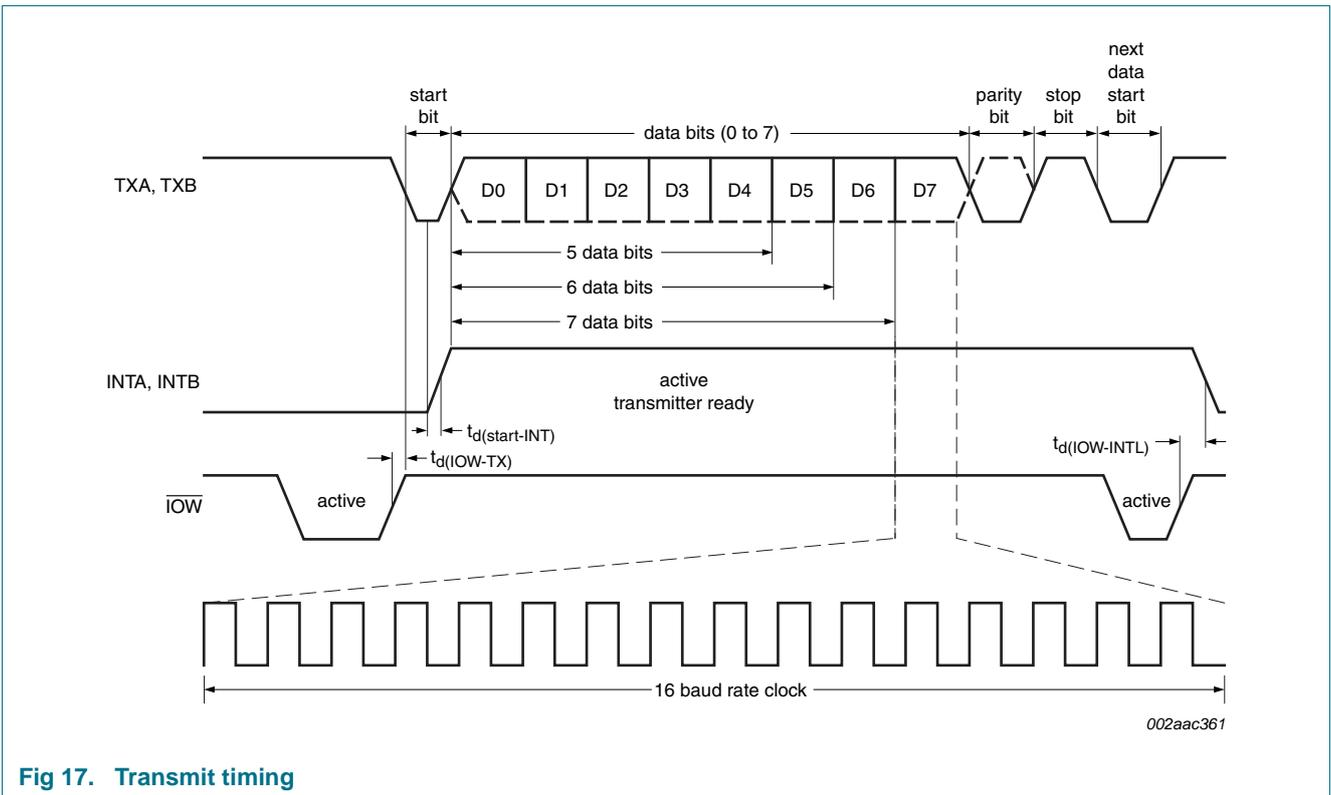
Fig 17. Transmit timing
