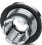
M12 threaded sleeve with tolerance-compensating function, for straight, SMD-solderable M12 socket contact inserts. Suitable for 1.6 mm ... 2.3 mm thick front plates.
