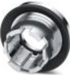
M12 threaded sleeve with tolerance-compensating function, for straight, SMD-solderable M12 socket contact inserts. Suitable for 0.9 mm ... 1.6 mm thick front plates.
