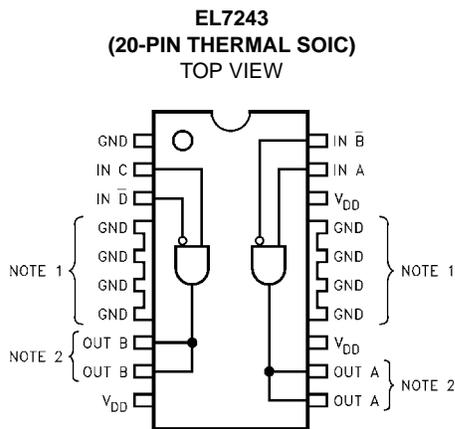
**Note 1:** Pins 4–7 and 14–17 are electrically connected.
