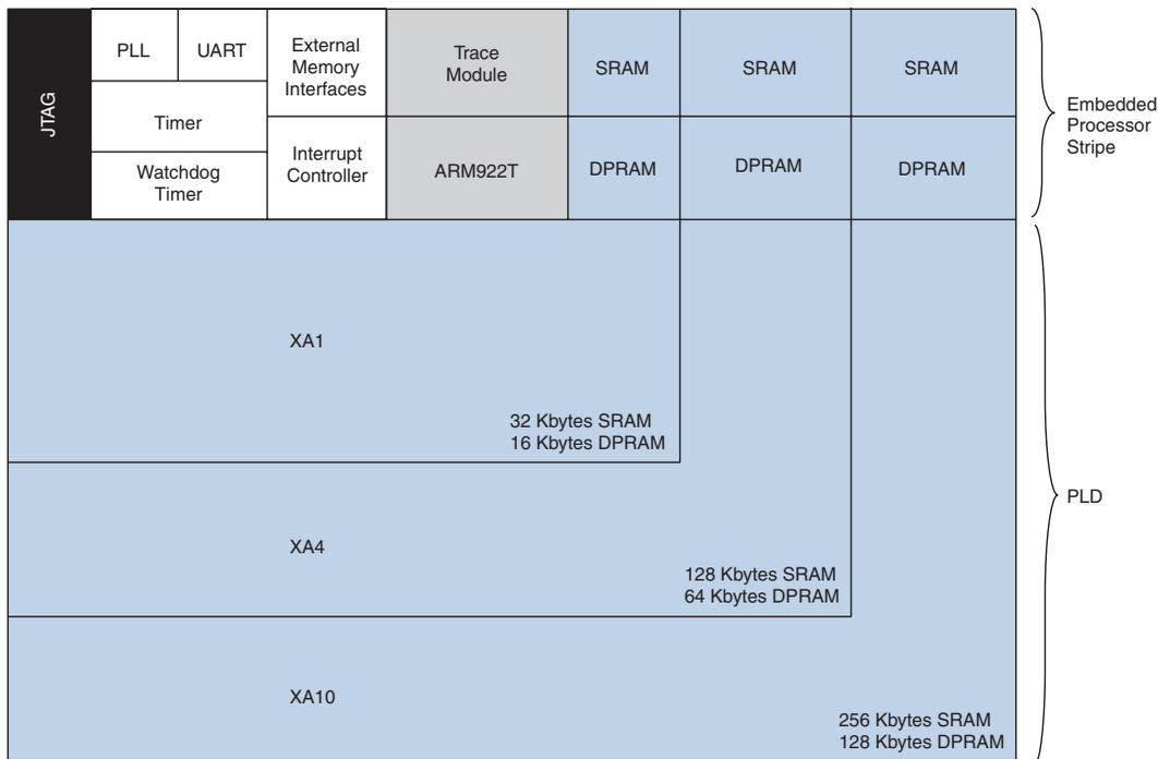
Figure 2. Excalibur System Architecture
