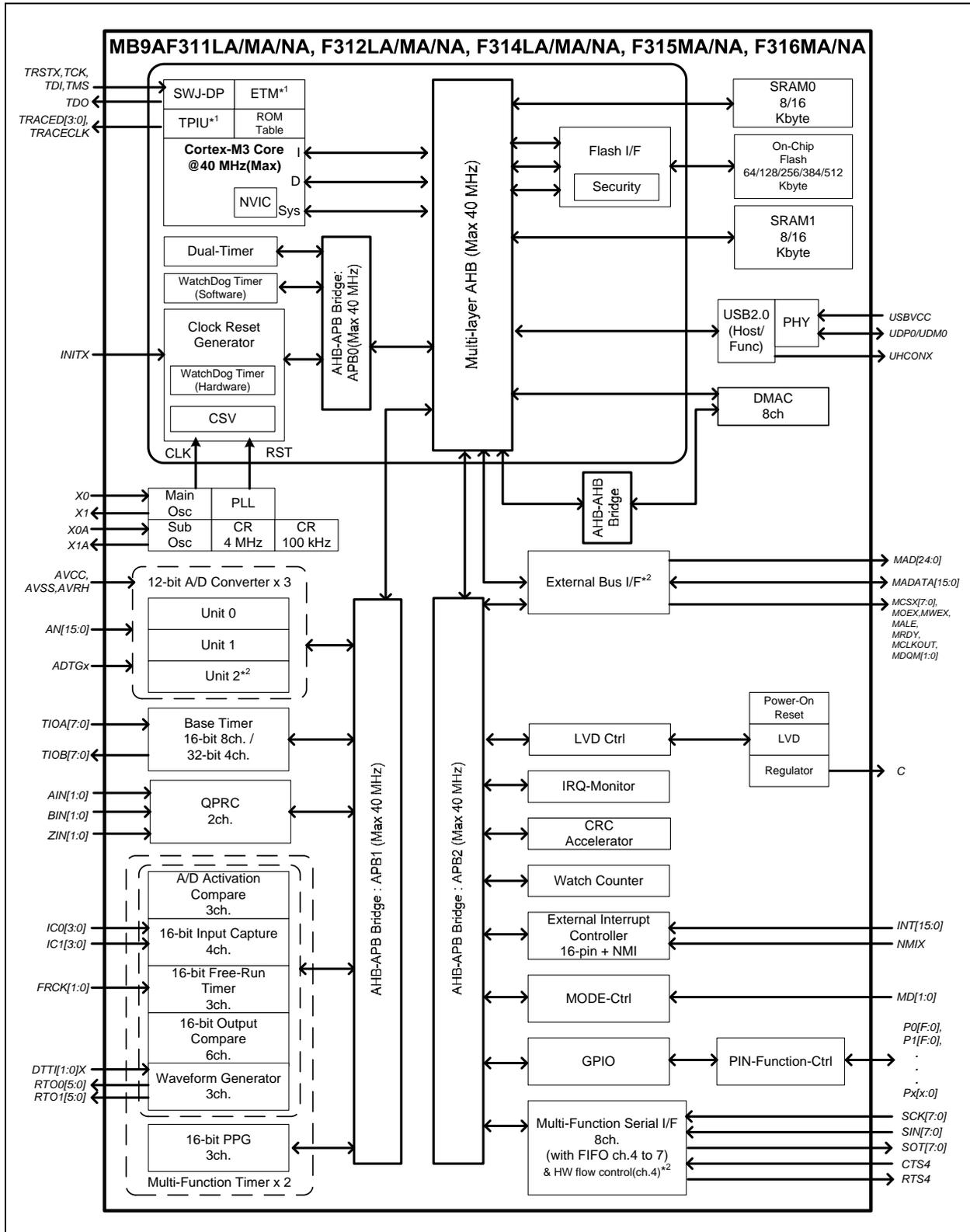
\*1: For the MB9AF311LA/MA, F312LA/MA, MB9AF314LA/MA, MB9AF315MA and MB9AF316MA, ETM is not available.
