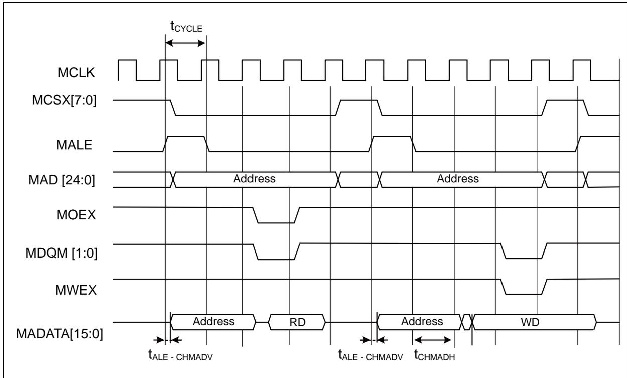
• Multiplexed Bus Access Synchronous SRAM Mode
