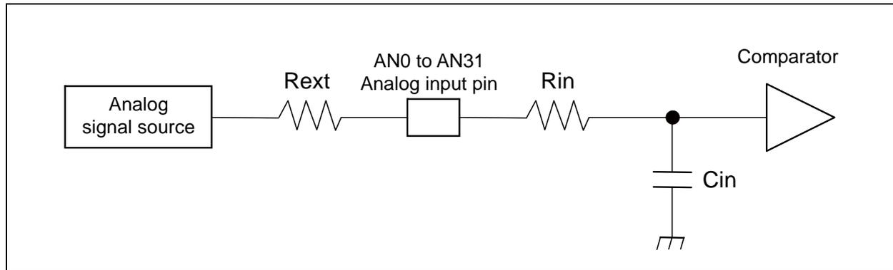
(Equation 1)  $T_s \geq (R_{in} + R_{ext}) \times C_{in} \times 9$
