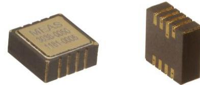
**The Model 3038** is a hermetically sealed SMD accelerometer designed for high performance applications. The accelerometer incorporates a gas-damped piezoresistive MEMS sensing element providing outstanding long-term stability. The model 3038 provides a millivolt output signal and features mechanical overload stops that provide shock protection to loads greater than 10,000g.
