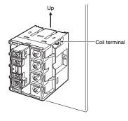
• Do not use the Relay with the terminal screw surfaces facing down.
