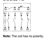
Note: The coil has no polarity.
