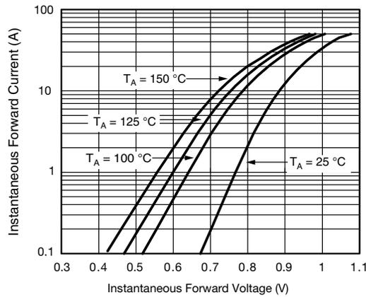
Fig. 4 - Typical Forward Characteristics Per Diode
