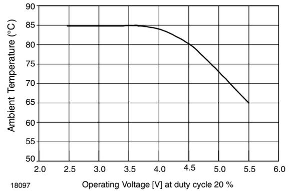
Figure 6. Temperature Derating Diagram
