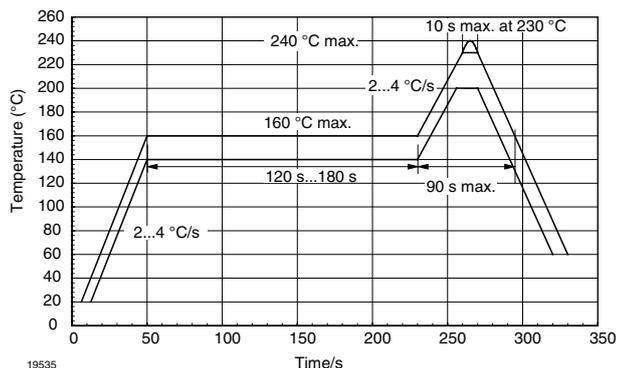
Figure 3. Recommended Solder Profile for Sn/Pb soldering
