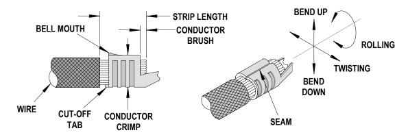
The above terminal drawing is a generic terminal representation. It is not an image of any terminal listed in the scope.
