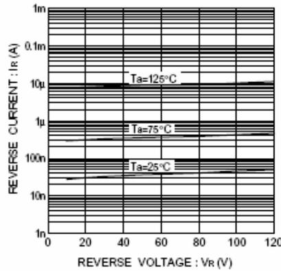
Fig.2 Reverse characteristics
