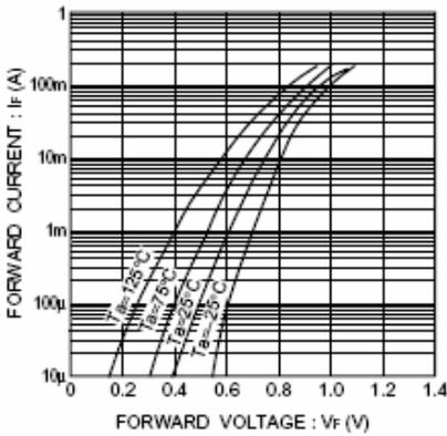
Fig.1 Forward characteristics
