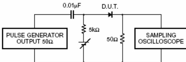
Fig.6 Reverse recovery time ( $t_r$ ) measurement circuit
