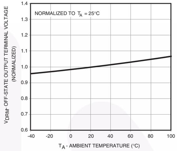
**Fig. 8 Off-State Output Terminal Voltage vs. Ambient Temperature**
