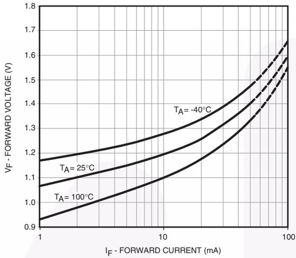
Fig. 3 LED Forward Voltage vs. Forward Current
