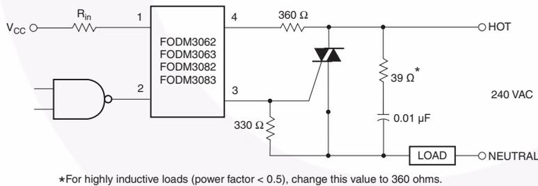
Typical circuit for use when hot line switching of 240 VAC is required. In this circuit the “hot” side of the line is switched and the load connected to the cold or neutral side. The load may be connected to either the neutral or hot line.
