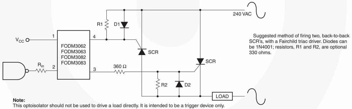
Figure 11. Inverse-Parallel SCR Driver Circuit (240 VAC)
