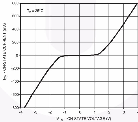
**Fig. 9 On-State Characteristics**
